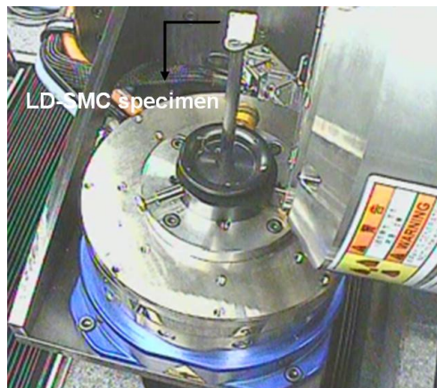
Fig. 1. Experimental setup of X-Ray micro-tomography (EasyTom nano)
