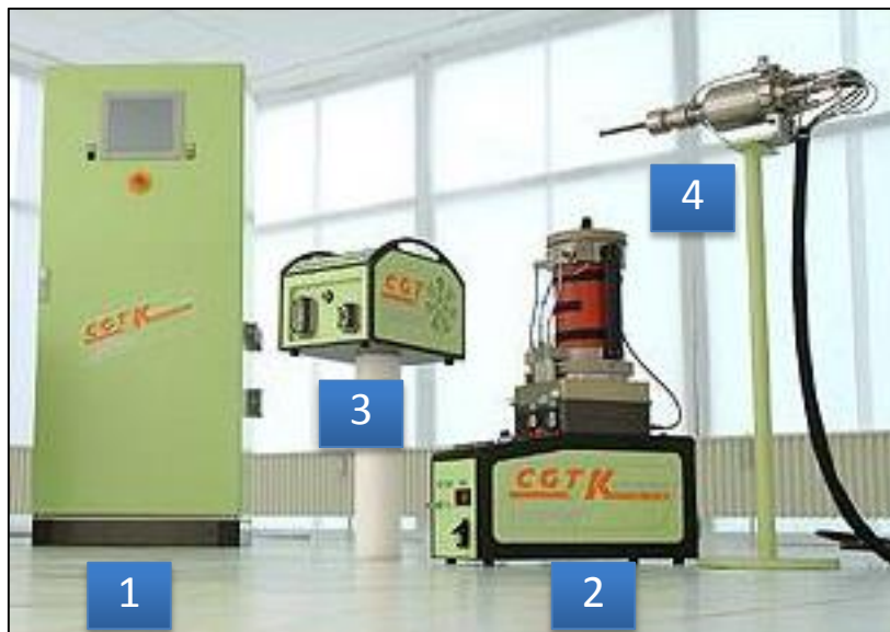
Figure II.1 : Equipement cold spray.
