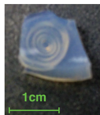
Figure 3-11: Photography of spiral cracks observed at the end of the drying process for samples drying on adhesive substrates.
