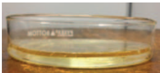
Figure 2-13: Picture of the petri dish (glass, 10cm outer diameter), containing the PDMS gel at the bottom and the birefringent polymer sheet on top (yellow color).
