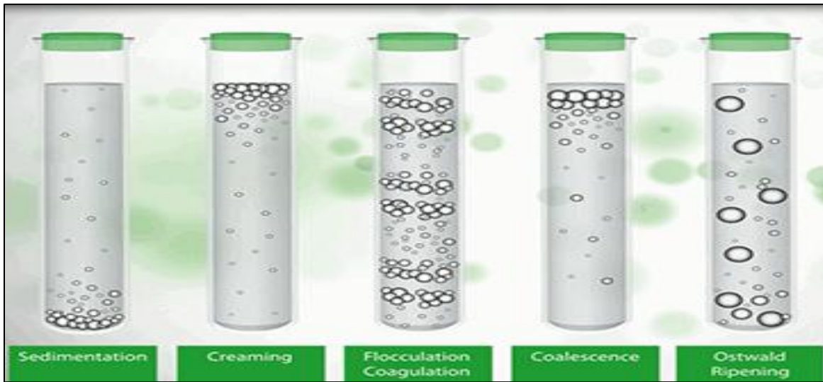
Figure 1.2.4: The main instability phenomena that can occur during emulsification
