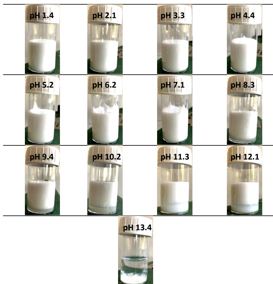
Figure 4.9: Effect of pH of the water phase on the stability of the Pickering O/W emulsions
