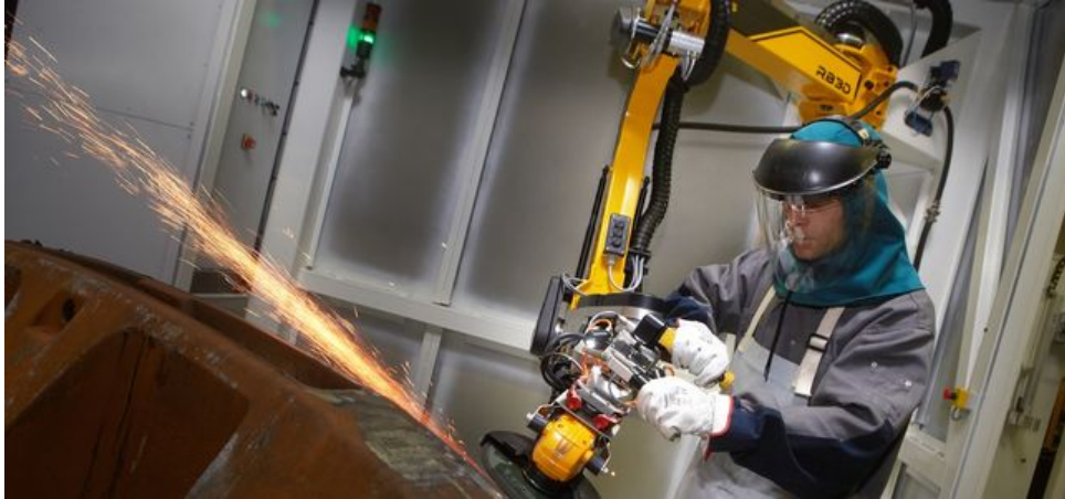
Figure 1.6: RB3D collaborative robot. This image shows an example of hands on interaction since the user directly manipulates the tool through the robot.
