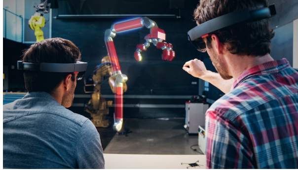
Figure 7.4: HoloLens for augmented reality. The use of augmented reality would improve the immersion of the user in the robot workspace. For example, the user could be able to visualize a preview of the robot movements before launching their execution.
