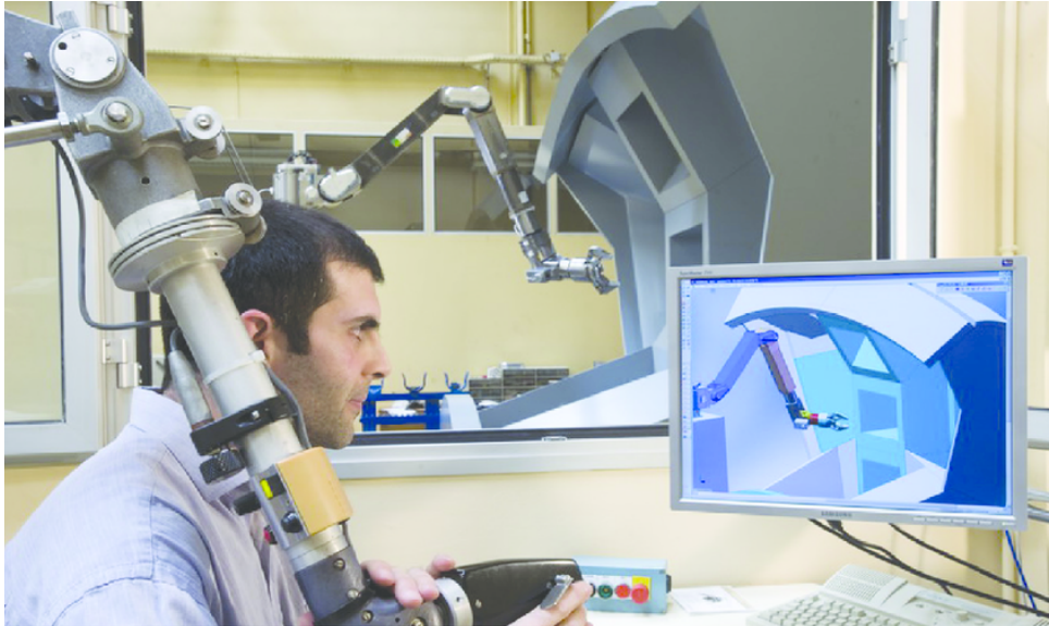
Figure 1.5: In [David et al., 2014] virtual guides are created on the fly into a physical engine, using linear interpolations. Since the guides are not programmed into the real robot controller, slight variations in their respective positions are possible. Also, in the context of co-manipulation tasks it would be more natural to program virtual guides in the real workspace rather than in a simulated one. This is one of the advantages of the hands on approach compared to the teleoperation.
