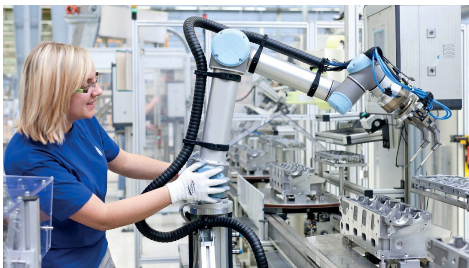
Figure 1.3: A cobot from Universal Robots working on a motor assembly.
