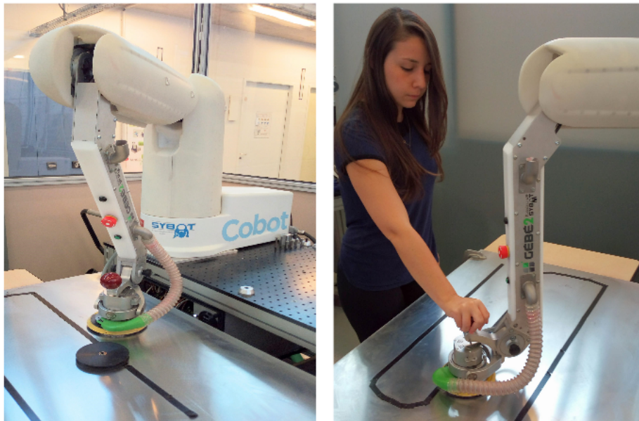
Figure 6.6: Left: ISybot robot with sanding tool and obstacle. Right: setup for the sanding experiment
