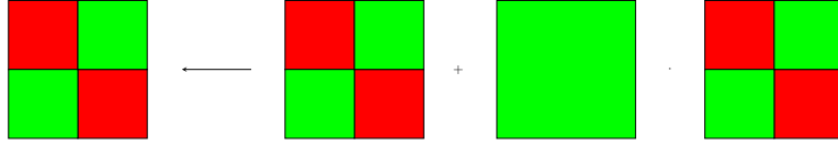
Figure 2.34: A_{\tau,\sigma} is an \mathcal{H} -matrix, A_{\tau,\zeta} is a low-rank matrix and A_{\zeta,\sigma} is an \mathcal{H} -matrix.
