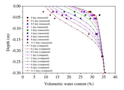
Figure 4. 13. Comparisons between the calculated and measured soil volumetric water content profiles at different moments in Test 1: *t* = 0 day, 0.2 day, 0.5 day, 1 day, 2 days, 4 days, 6 days, 8 days and 11.5 days
