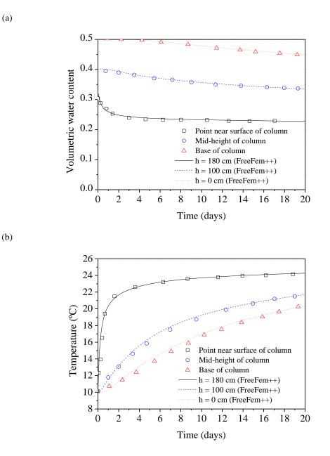
Figure 2. 8. Comparisons of computation results by two methods in Case 2: (a) volumetric moisture content variations at different positions; (b) temperature variations at different positions
