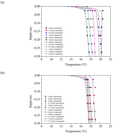
Figure 4. 16. Comparisons between the calculated and measured soil temperature profiles at different moments in Test 3: (a) t = 0 day, 0.2 day, 0.5 day, 1 day, 4 days, and 6 days; (b) t = 4 days, 6 days, 8 days, 11.5 days, 15 days, and 17.5 days
