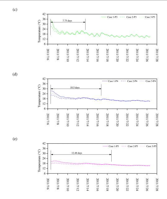
Figure 5. 28. Soil temperature variations with soil thermal conductivity  $\lambda = \lambda_{\text{original}}+1$  in the three cases with different initial temperatures: (a) at point P1; (b) at point P2; (c) at point P3; (d) at point P4; (e) at point P5
