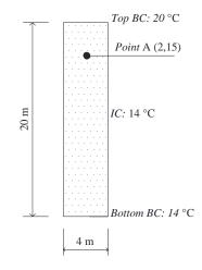
Figure 2. 1. Model details for heat flow in soil
