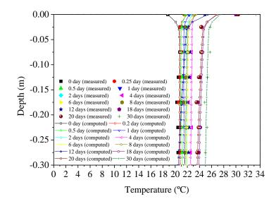
Figure 4. 18. Comparisons between the calculated and measured soil temperature profiles at different moments in Test 4: t = 0 day, 0.25 day, 0.5 day, 1 day, 2 days, 4 days,
