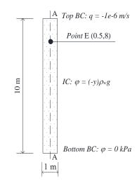
Figure 2. 3. Model details for the verification of water flow in soil
