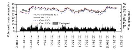
Figure 6. 35. Calculated soil volumetric water content variations in Case 1, Case 4, Case 5 and measured data of point 3C4 along with wind speed information
