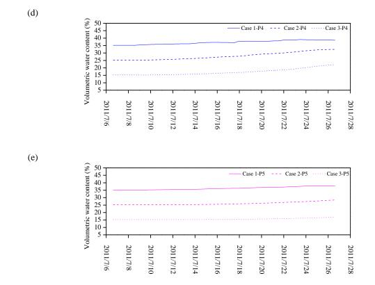
Figure 5. 33. Soil volumetric water content variations in the three cases with different initial volumetric water content conditions: (a) at point P1; (b) at point P2; (c) at point P3; (d) at point P4; (e) at point P5
