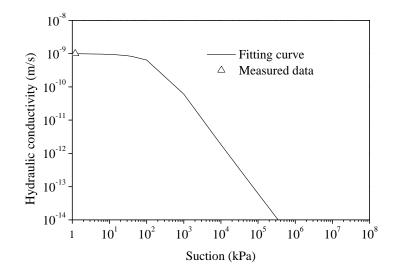
Figure 6.8. Hydraulic conductivity curve versus suction for the silt treated by 2% CaO
