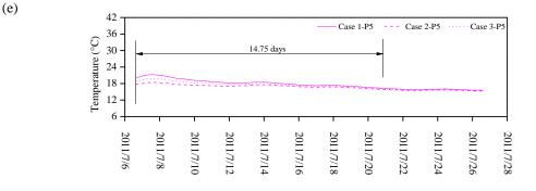
Figure 5. 27. Soil temperature variations with soil thermal conductivity  $\lambda = \lambda_{\text{original}} + 0.5$  in the three cases with different initial temperatures: (a) at point P1; (b) at point P2; (c) at point P3; (d) at point P4; (e) at point P5
