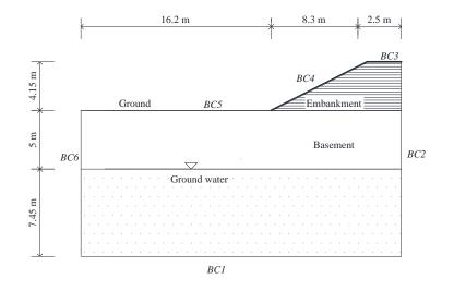
Figure 5. 16. Numerical model dimensions for Héricourt embankment
