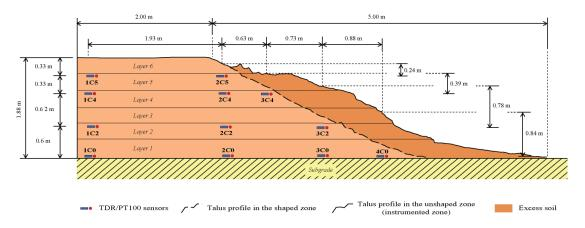
Figure 6. 4. Field instrumentation profile of Rouen embankment, providing information about the number and position of each sensor
