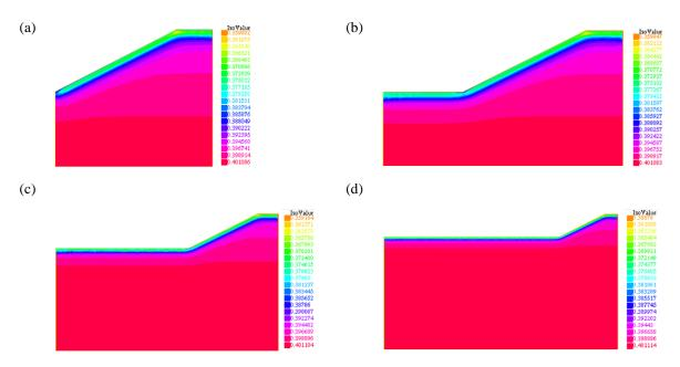
Figure 5. 12. Volumetric water content distributions in the four dimensions at day 6: (a) Dimensions 1; (b) Dimensions 2; (c) Dimensions 3; (d) Dimensions 4
