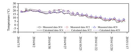
Figure 6. 14. Soil temperature comparisons between the calculation and measurement for points 3C4, 3C2 and 4C0 during the studied period
