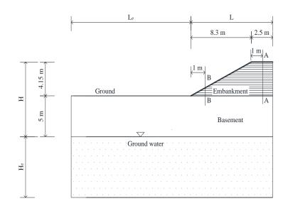
Figure 5. 9. Héricourt embankment dimension
