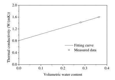
Figure 6. 6. Thermal conductivity curve versus volumetric water content for the silt
