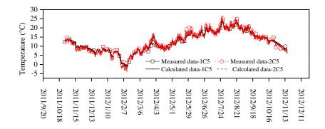
Figure 6. 21. Soil temperature comparisons between the simulation results and measurement data of points 1C5 and 2C5 during the studied period
