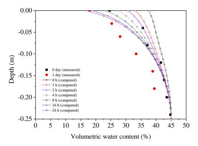
Figure 3. 12. Comparisons of soil volumetric water content between the calculated and measured results at different moments: t = 0 h, 1 h, 2 h, 4 h, 8 h, 16 h, and 24 h for computed results; t = 0 h and 24 h for measured results
