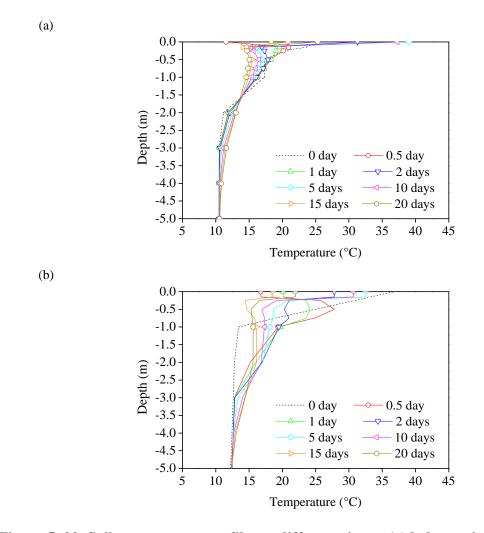
Figure 5. 22. Soil temperature profiles at different times: (a) below point A1; (b) below point A2
