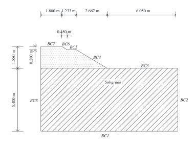
Figure 6. 9. Model dimensions adopted for Rouen embankment
