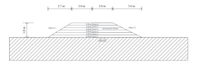
Figure 6. 3. Cross section of Rouen embankment
