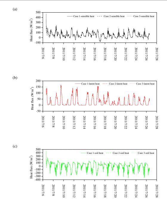
Figure 5. 26. Heat flux variations during the studied time period: (a) sensible heat; (b) latent heat; (c) soil heat
