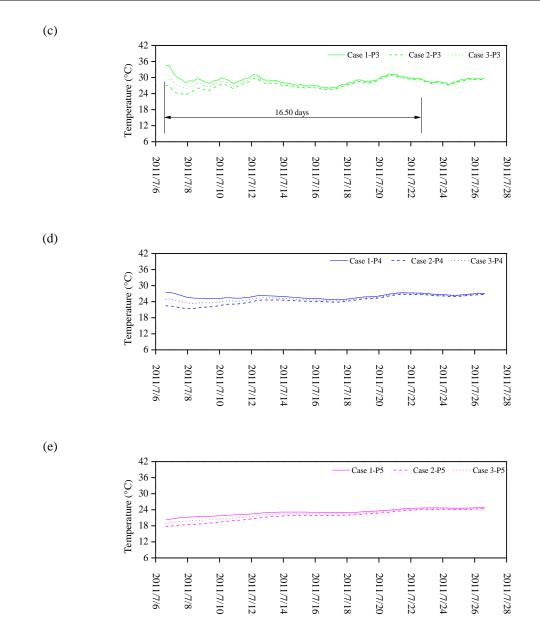
Figure 5. 30. Soil temperature variations when the time step is six hours: (a) at point P1; (b) at point P2; (c) at point P3; (d) at point P4; (e) at point P5
