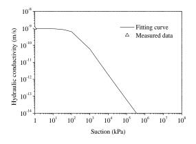
Figure 5. 8. Hydraulic conductivity curve versus suction for the treated silt
