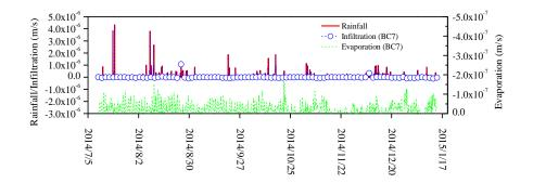
Figure 6. 11. Water fluxes at the top surface of Rouen embankment (BC7): rainfall, infiltration, and evaporation
