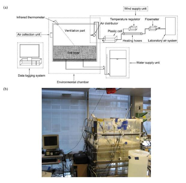
Figure 4. 1. (a) Sketch of the environmental chamber test system; (b) Outlook of the environmental chamber system (Song at al. 2014)
