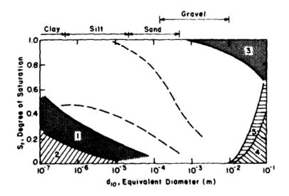
Figure 1. 3. Regions of predominant influence of various heat transfer mechanisms against soil grain size and degree of saturation. Expected variations in degree of saturation under field condition lie in the region bounded by dashed lines (after Johansen 1975 and Farouki 1981): 1-thermal redistribution of moisture; 2-vapor diffusion due to moisture gradient; 3-free convection in water; 4-free convection in air; 5-heat radiation (Farouki 1981)
