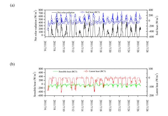
Figure 5. 17. Heat fluxes at the top surface of Héricourt embankment (BC3): (a) net solar radiation and soil heat; (b) sensible heat and latent heat
