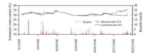
Figure 6. 29. Comparison of soil volumetric water content variations between the simulated and measured data of point 3C4 along with rainfall information (187 days)
