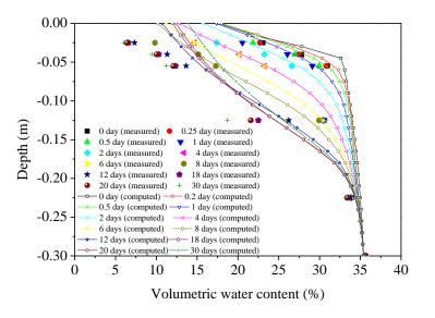
Figure 4. 19. Comparisons between the calculated and measured soil volumetric water content profiles at different moments in Test 4: *t* = 0 day, 0.25 day, 0.5 day, 1 day, 2 days, 4 days, 6 days, 8 days, 12 days, 18 days, 20 days, and 30 days
