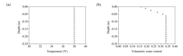
Figure 3. 6. The initial conditions of (a) soil temperature and (b) volumetric water
