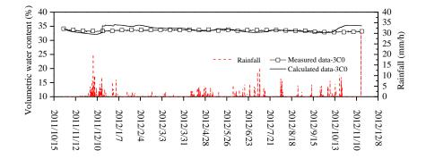
Figure 6. 33. Comparison of soil volumetric water content variations between the simulated and measured data of point 3C0 along with rainfall information (387 days)
