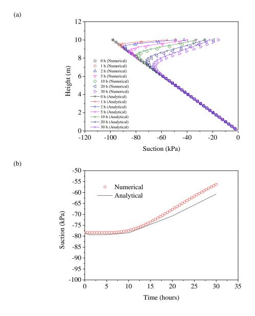
Figure 2. 5. Comparison between numerical and analytical methods: (a) soil suction profile at section A at different moments: *t* = 1 h, 2 h, 5 h, 10 h, 20 h, 30 h; (b) soil suction variation at point E (0.5, 8)
