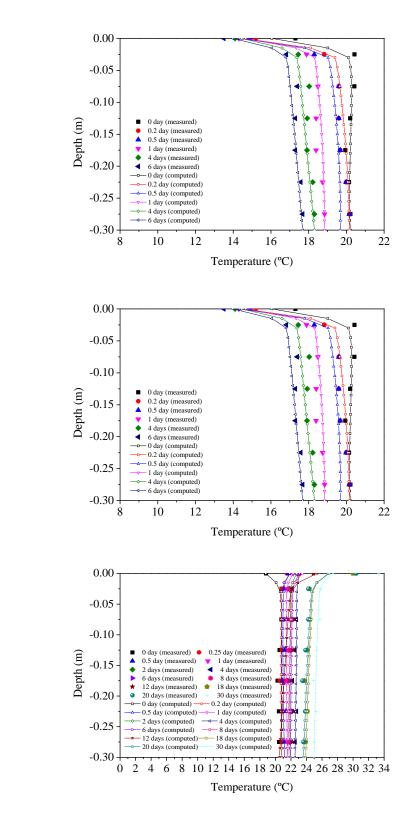
Figure 4. 25. Comparisons of soil temperature between the measured and calculated results at different moments: (a) Test 1; (b) Test 2; (c) Test 3; (d) Test 4.
