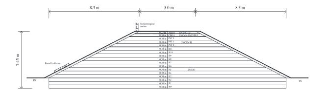
Figure 5. 4. Studied cross section of Héricourt embankment with soil treatment information
