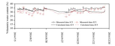
Figure 6. 17. Soil volumetric water content comparisons between the simulation results and measurement data of points 1C5 and 2C5 during the studied period
