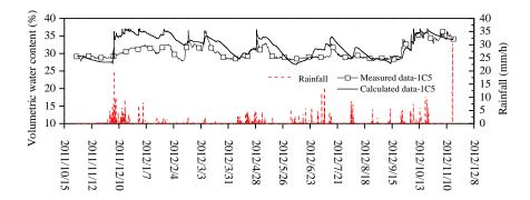
Figure 6. 31. Comparison of soil volumetric water content variations between the simulated and measured data of point 1C5 along with rainfall information (387 days)
