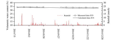
Figure 6. 30. Comparison of soil volumetric water content variations between the simulated and measured data of point 3C0 along with rainfall information (187 days)
