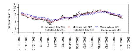
Figure 6. 23. Soil temperature comparisons between the simulation results and measurement data of points 2C4, 2C2 and 2C0 during the studied period
