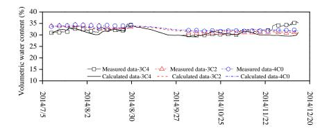
Figure 6. 18. Soil volumetric water content comparisons between the simulation results and measurement data of points 3C4, 3C2 and 4C0 during the studied period
