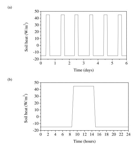
Figure 5. 13. In Case 2: (a) heat flux conditions on the top boundaries in six days; (b) details of the heat flux variations in 24 hours
