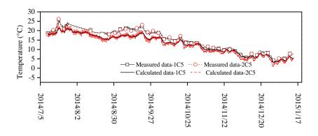
Figure 6. 13. Soil temperature comparisons between the calculation and measurement
