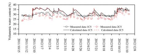
Figure 6. 25. Soil volumetric water content comparisons between the simulation results and measurement data of points 1C5 and 2C5 during the studied period
