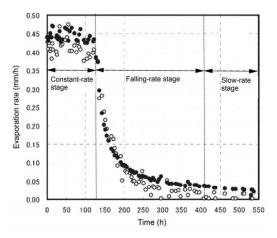
Figure 4. 21. The general three stages of evaporation process (Qiu and Ben-Asher 2010)
