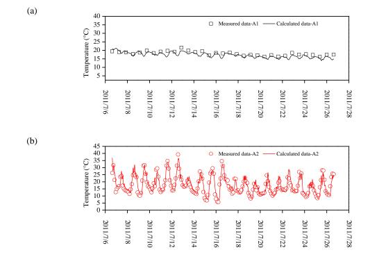
Figure 5. 21. Temperature comparisons between the measured data and simulation data: (a) for slope surface point A1; (b) for top surface point A2
