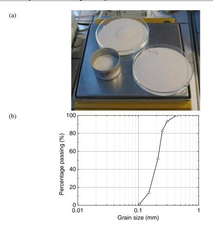
Figure 4. 4. Fontainebleau sand: (a) picture of Fontainebleau sand; (b) grain size distribution curve
