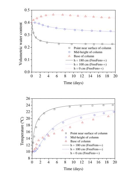
Figure 2. 7. Comparisons of the computation results by two methods in Case 1: (a) volumetric moisture content variations at different positions; (b) temperature variations at different positions
