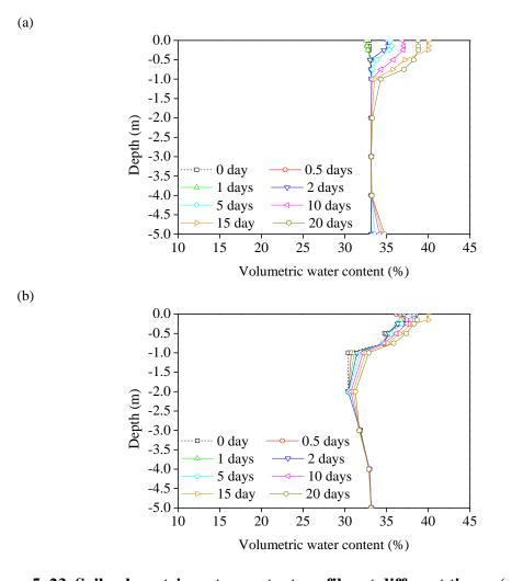
Figure 5. 23. Soil volumetric water content profiles at different times: (a) below point A1; (b) below point A2
