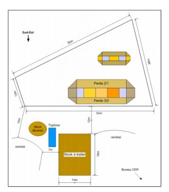
Figure 6. 1. Field site plan of Rouen experimental embankment
