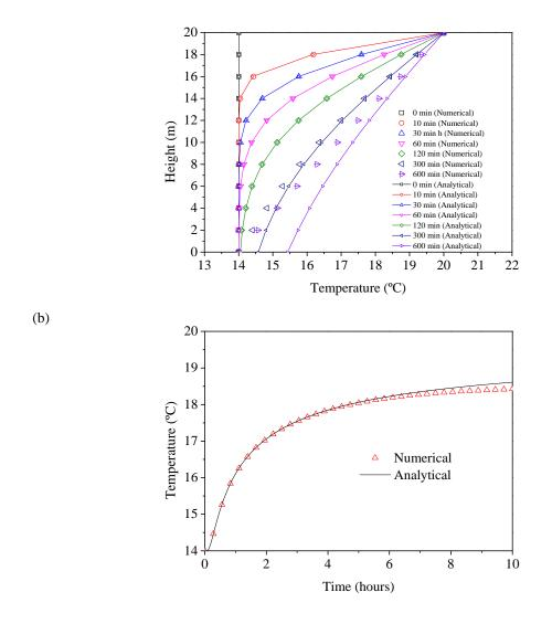
Figure 2. 2. Comparison of soil temperature between numerical simulation and analytical solution: (a) soil temperature profiles at different moments: t = 0, 10 min, 30 min, 60 min, 120 min, 300 min, 600 min; (b) soil temperature variation over time at Point A (2, 15)
