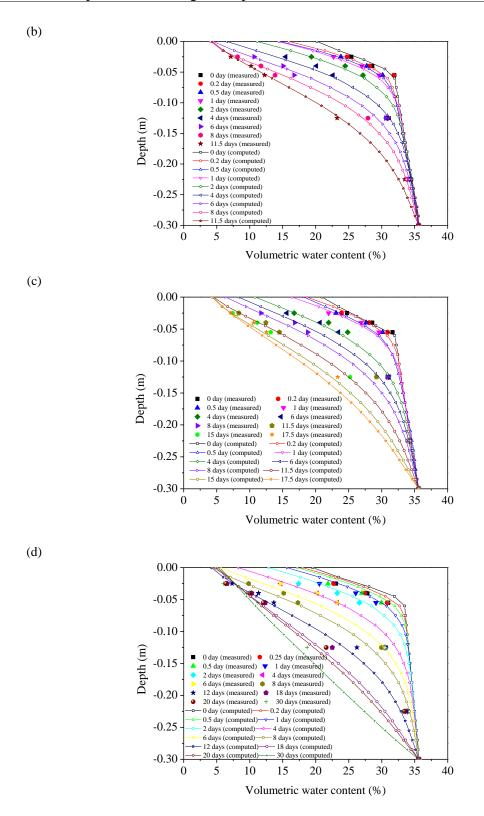
Figure 4. 26. Comparison of soil volumetric water content between the measured and calculated results at different moments: (a) Test 1; (b) Test 2; (c) Test 3; (d) Test 4
