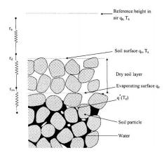
Figure 3. 2. The three stages of water vapor transportation from soil to atmosphere (Aluwihare and Watanabe 2003)
