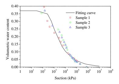
Figure 6. 7. Water retention curve versus suction for the silt treated by 2% CaO
