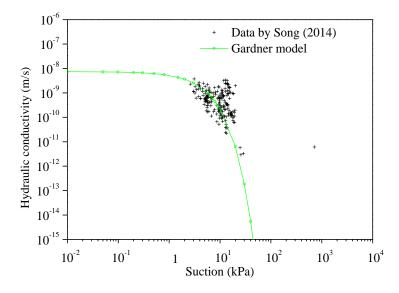
Figure 4. 24. Soil hydraulic conductivity curve versus suction based on Gardner model
