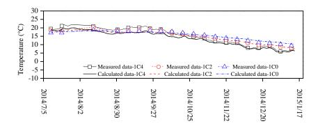
Figure 6. 16. Soil temperature comparisons between the simulation results and measurement data of points 1C4, 1C2 and 1C0 during the studied period
