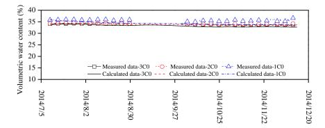
Figure 6. 19. Soil volumetric water content comparisons between the simulation results
