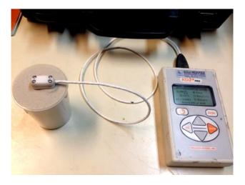
Figure 4. 7. KD2 Analyzer used to measure thermal conductivity for Fontainebleau sand
