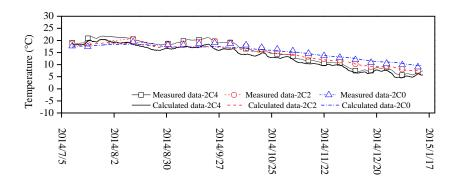
Figure 6. 15. Soil temperature comparisons between the simulation results and measurement data of points 2C4, 2C2 and 2C0 during the studied period
