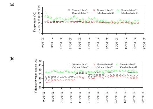
Figure 5. 20. Comparisons between the measured data and calculated data for the near soil surface points S1, S2, and S3: (a) temperature variations; (b) volumetric water content variations
