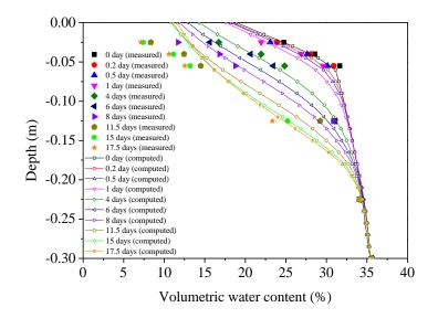
Figure 4. 17. Comparisons between the calculated and measured soil volumetric water content profiles at different moments in Test 3: t = 0, 0.2 day, 0.5 day, 1 day, 4 days, 6 days, 8 days, 11.5 days, 15 days, and 17.5 days
