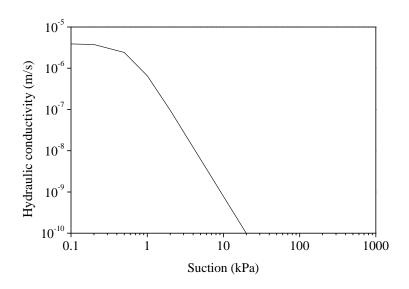
Figure 3. 10. Hydraulic conductivity curve versus suction for Beaver Creek sand
