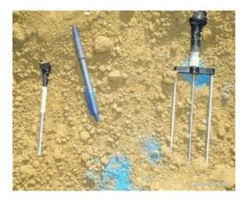
Figure 6. 5. PT100 sensor for soil temperature measurement (left) and TDR sensor for soil volumetric water content measurement (right)
