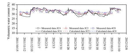
Figure 6. 26. Soil volumetric water content comparisons between the simulation results and measurements data of points 3C4, 3C2 and 4C0 during the studied period
