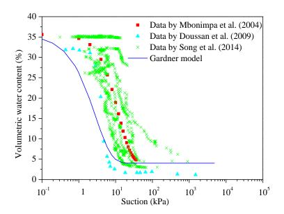
Figure 4. 23. Soil water retention curve versus suction based on Gardner model
