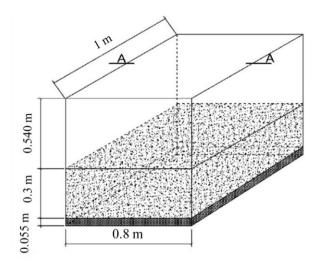
Figure 4. 2. Three-dimensional view of the environmental chamber (Song at al. 2014)
