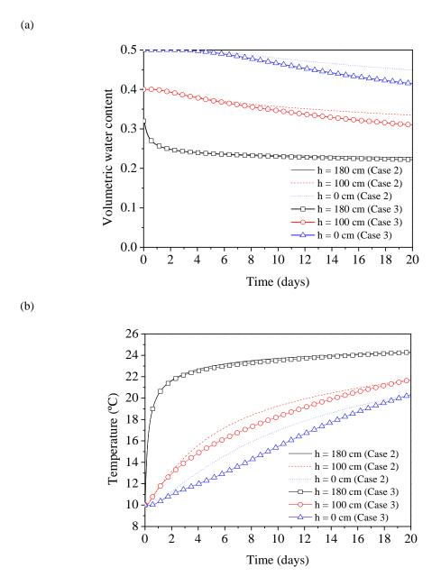
Figure 2. 10. Comparisons of computation results for the three studied points in Case 2 and Case 3: (a) volumetric moisture content variations over time; (b) temperature variations over time
