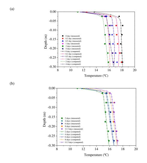
Figure 4. 12. Comparisons between the calculated and measured soil temperature profiles at different moments in Test 1: (a) t = 0 day, 0.2 day, 0.5 day, 1 day, 2 days, 4 days; (b) t = 2 days, 4 days, 6 days, 8 days, 11.5 days
