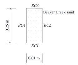
Figure 3. 5. Model dimensions of column drying test
