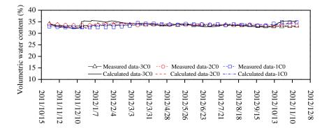
Figure 6. 27. Soil volumetric water content comparisons between the simulation and measurement for points 3C0, 2C0 and 1C0 during the studied period
