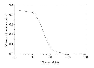
Figure 3. 9. Water retention curve for Beaver Creek sand
