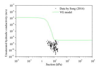
Figure 4. 11. Hydraulic conductivity curve versus suction for Fontainebleau sand
