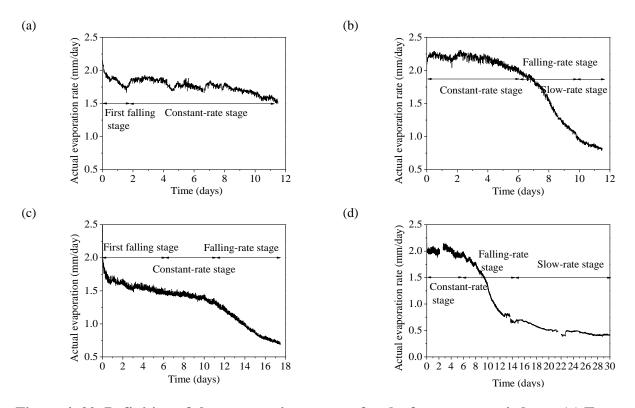
Figure 4. 20. Definition of the evaporation process for the four tests carried out: (a) Test
