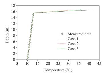
Figure 5. 24. Soil temperature measurement profile and assumed three initial soil temperature conditions below point A2
