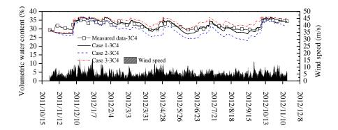
Figure 6. 34. Calculated soil volumetric water content variations in Case 1, Case 2, Case 3 and measured data of point 3C4 along with wind speed information
