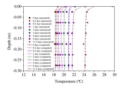
Figure 4. 14. Comparisons between the calculated and measured soil temperature profiles at different moments in Test 2: t = 0 day, 0.2 day, 0.5 day, 1 day, 2 days, 4 days,
