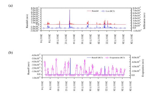
Figure 5. 18. Water fluxes at the top surface of Héricourt embankment (BC3): (a) rainfall and infiltration; (b) runoff and evaporation
