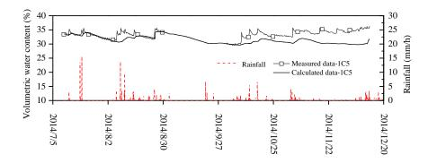
Figure 6. 28. Comparison of soil volumetric water content variations between the simulated and measured data of point 1C5 along with rainfall information (187 days)
