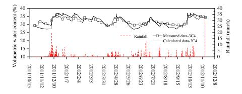
Figure 6. 32. Comparison of soil volumetric water content variations between the simulated and measured data of point 3C4 along with rainfall information (387 days)
