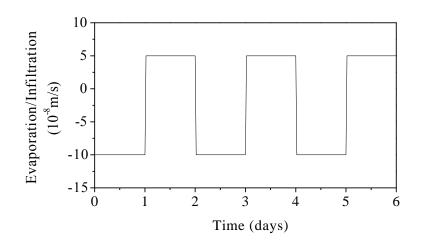
Figure 5. 10. Water flux conditions on the top boundaries in six days in Case 1
