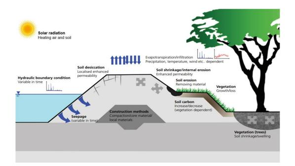
Figure 1. 2. The interactions between geotechnical infrastructure and climate (after Vardon 2015)
