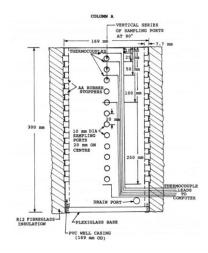
Figure 3. 4. Details about drying test of column A (Wilson 1990)
