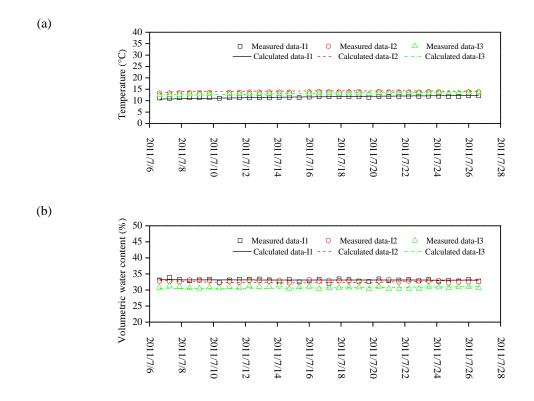
Figure 5. 19. Comparisons between the measured data and calculated data for interior points I1, I2, and I3: (a) temperature variations; (b) volumetric water content variations
