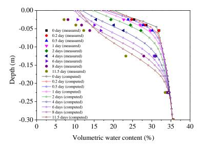
Figure 4. 15. Comparisons between the calculated and measured soil volumetric water content profiles at different moments in Test 2: *t* = 0 day, 0.2 day, 0.5 day, 1 day, 2 days, 4 days, 6 days, 8 days, and 11.5 days
