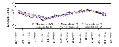
Figure 6. 24. Soil temperature comparisons between the simulation results and measurement data of points 1C4, 1C2 and 1C0 during the studied period
