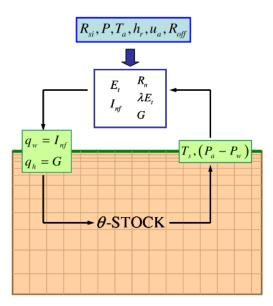
Figure 1. 6. The flow chart of  $\theta$ -STOCK code (Hemmati et al. 2012)
