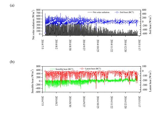
Figure 6. 10. Heat fluxes at the top surface of Rouen embankment (BC7): (a) net solar radiation and soil heat; (b) sensible heat and latent heat
