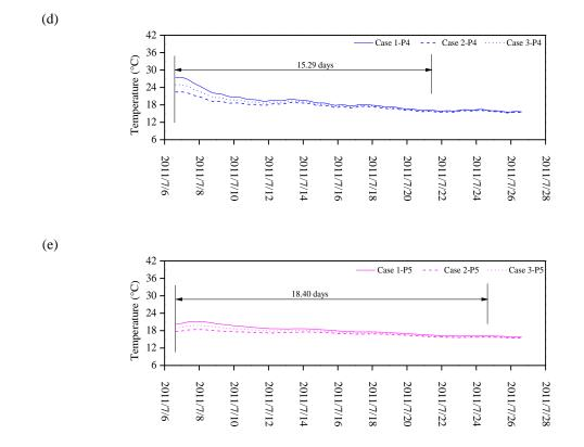
Figure 5. 25. Soil temperature variations in the three cases with different initial temperature conditions: (a) at point P1; (b) at point P2; (c) at point P3; (d) at point P4; (e) at point P5
