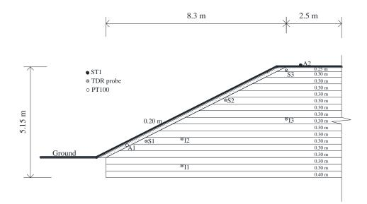
Figure 5. 3. Embankment instrumentation: TDR sensors for recording soil volumetric water content variations and temperature variations (I1~3, S1~3) in the embankment;
