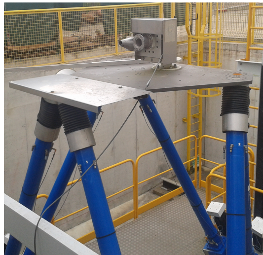
Figure 1.17: The scaled manifold on its hexapod.
