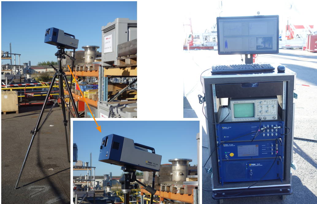
Figure 3.1: The laser vibrometer measures the velocity of all measurement points of the mesh. Left and bottom pictures: Head of the laser vibrometer. Right picture: Acquisition and generation system.
