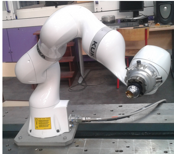
Figure 2.7: Picture of the robot during the measurements stage. A spherical reflector associated with the laser tracker is installed on the tip of the robot.
