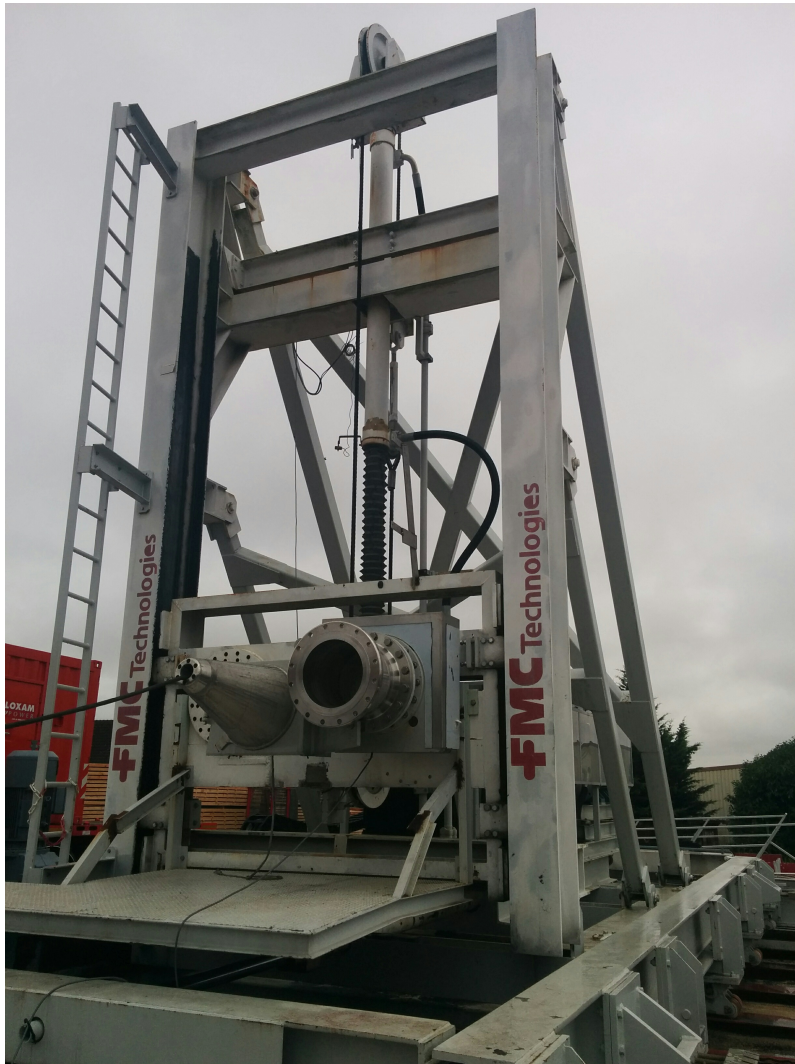
Figure 1.19: 3 DoF test bench is fitted with a manifold.
