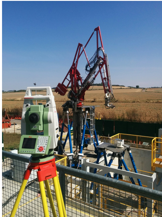
Figure 2.15: The total station measures the position of the coupler. Picture of the OLAF scaled model.
