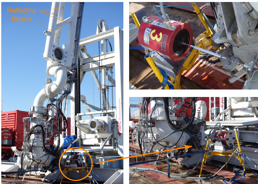
Figure 3.3: The excitator excites the structure of the arm via the coupler, and the transmitted force is calculated from the current in the coil.
