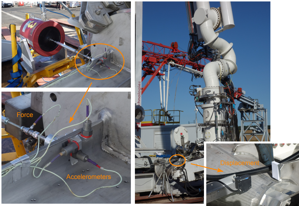
Figure 3.4: Pictures of the sensors set up at the excitement point.
