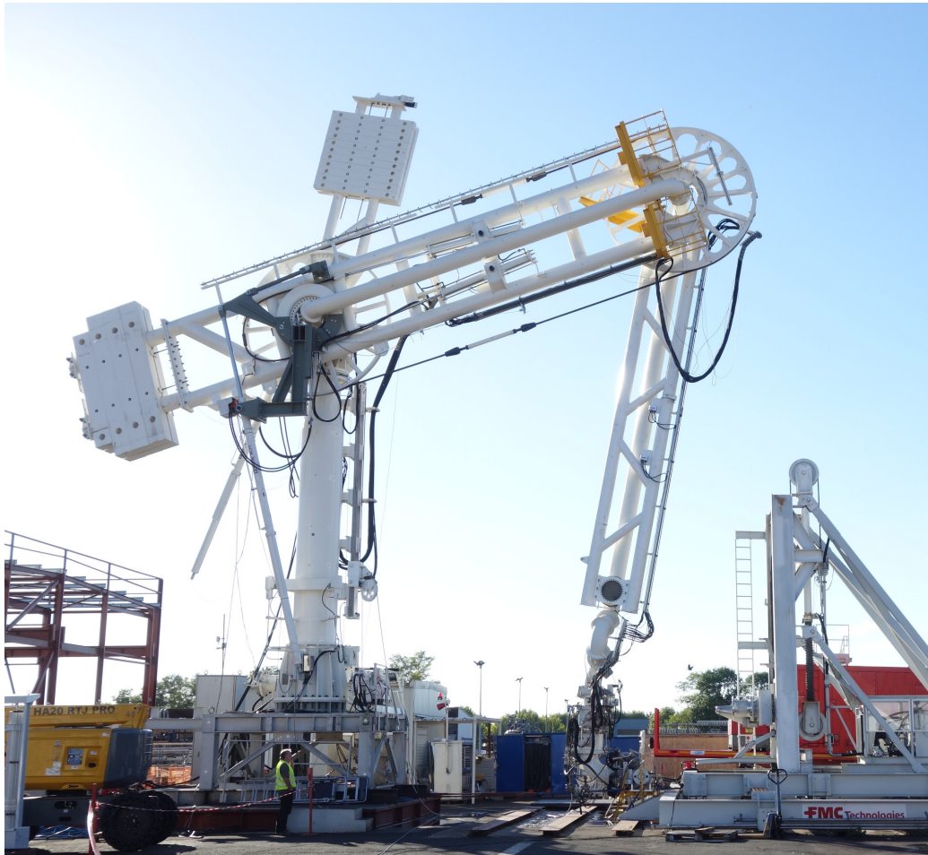
Figure 1.18: A full scale marine loading arm is used for the final tests of automatic connection.
