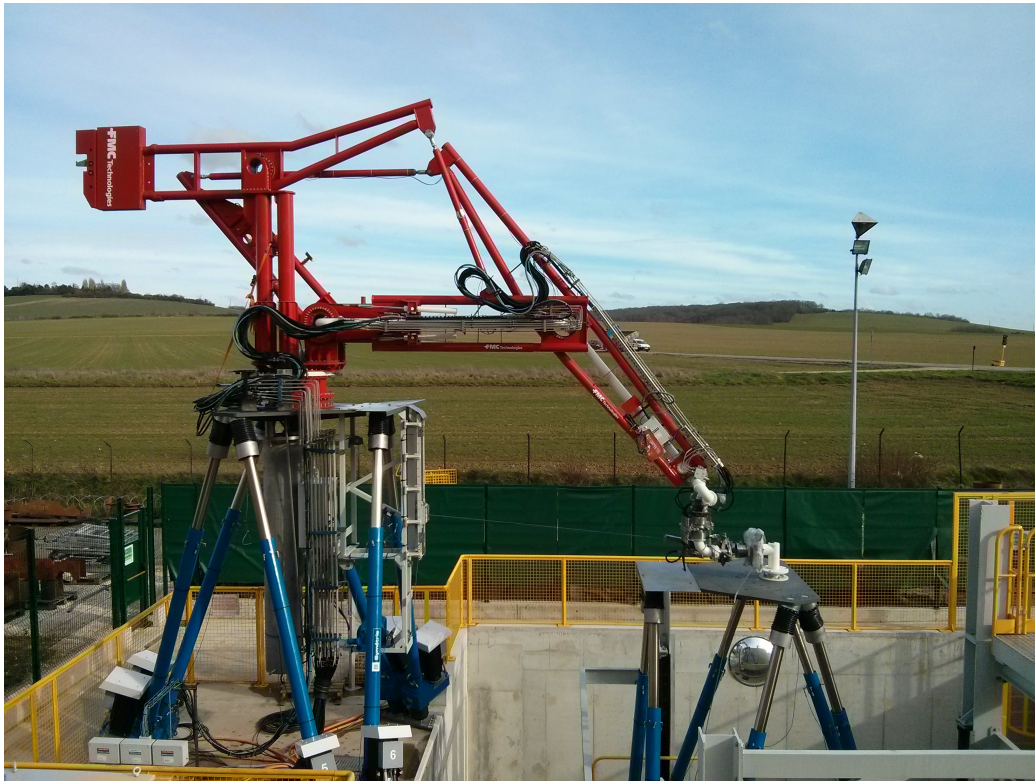
Figure 1.16: The OLAF scaled model connected to the manifold.
