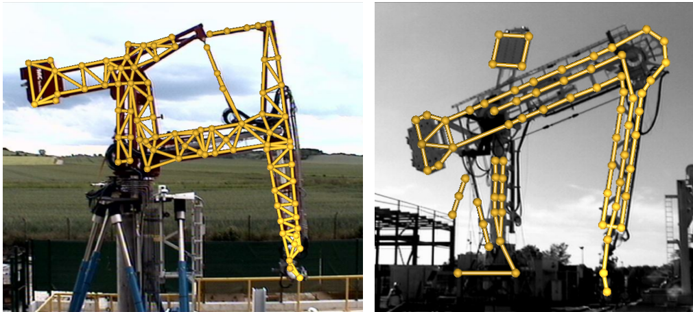
Figure 3.2: The structures of the scaled model and the full-scale loading arm are meshed with measurement points.
