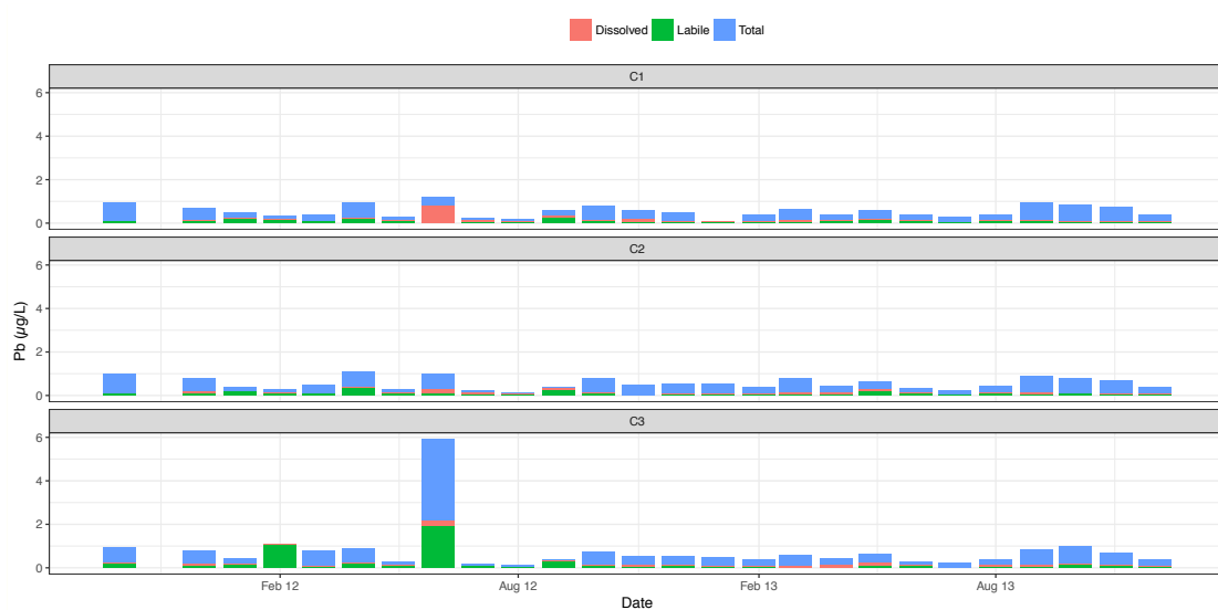
Figure 71 Total, dissolved and labile concentration of Pb at the points C1, C2, C3 of Lake Créteil. The labile concentration is in green. The dissolved concentration is the sum of green and red bars and the total concentration is the sum of the green, red and blue bars.
