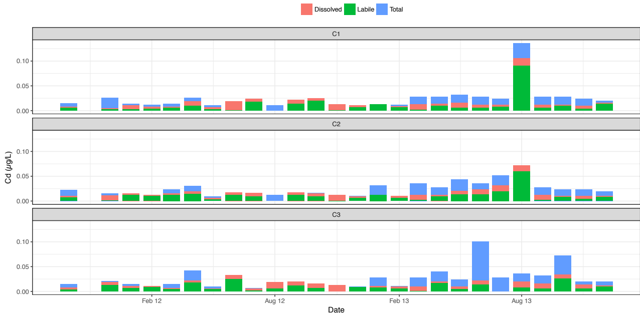
Figure 61 Total, dissolved and labile concentration of Cd at the points C1, C2, C3 of Lake Créteil. The labile concentration is in green. The dissolved concentration is the sum of green and red bars and the total concentration is the sum of the green, red and blue bars
