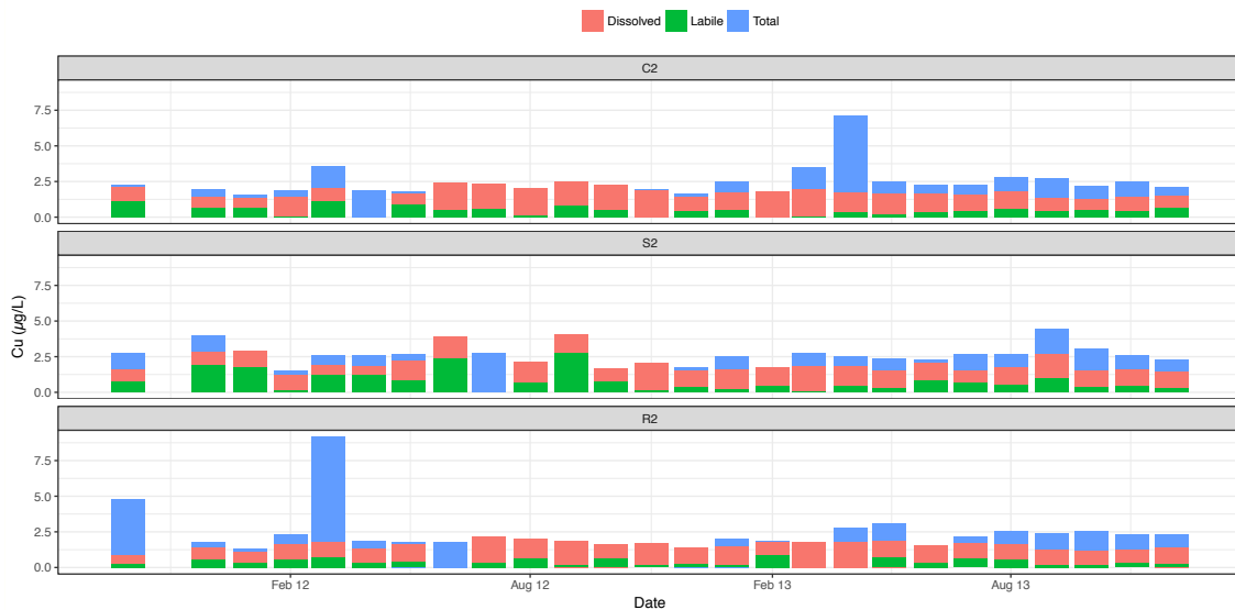
Figure 68 Total, dissolved and labile concentration of Cu at the points S2, C2, R2 of Lake Créteil. The labile concentration is in green. The dissolved concentration is the sum of green and red bars and the total concentration is the sum of the green, red and blue bars
