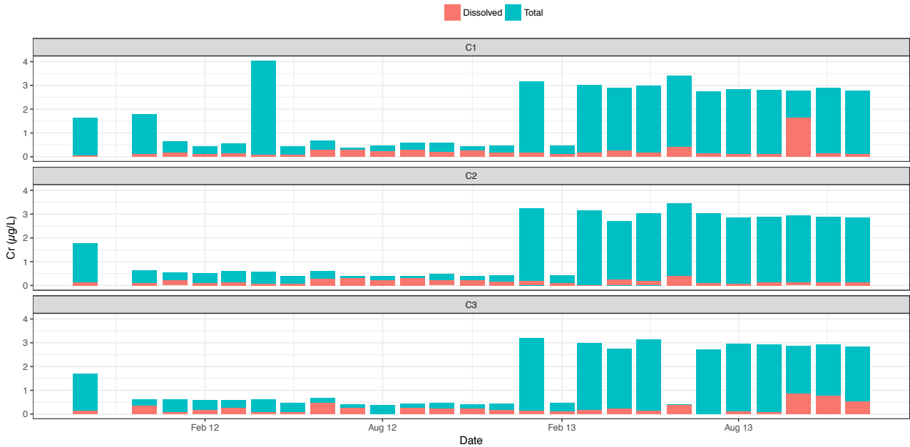
Figure 59 Total and dissolved concentration of Cr at the points C1, C2, C3 of Lake Créteil. The dissolved concentration is in red. The total concentration corresponds to the red + blue bar.
