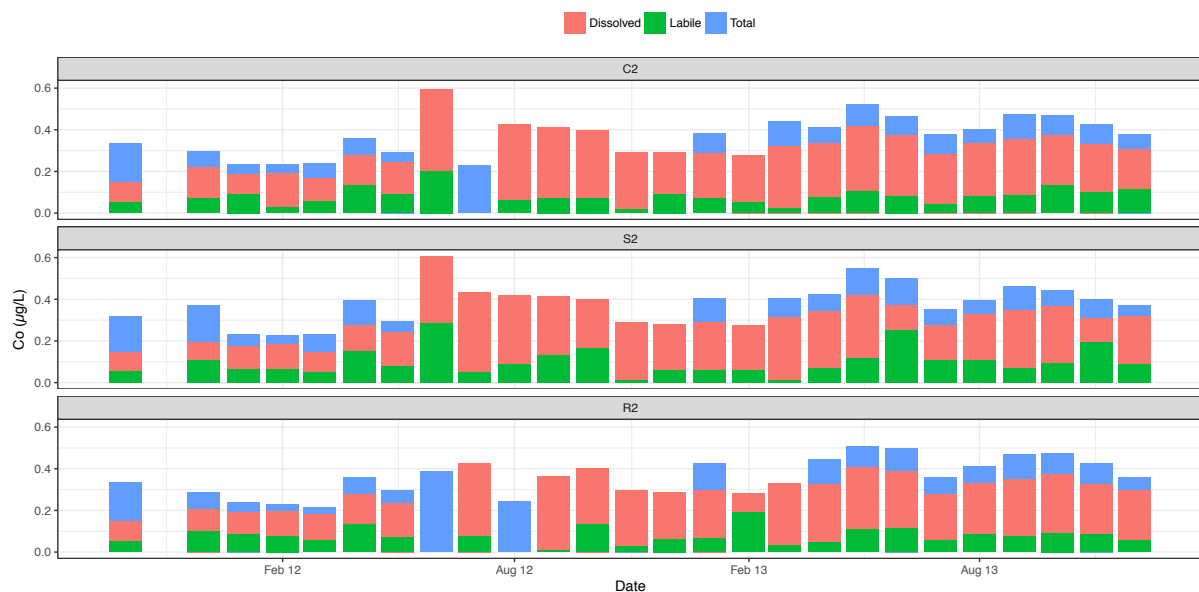
Figure 64 Total, dissolved and labile concentration of Co at the points S2, C2, R2 of Lake Créteil. The labile concentration is in green. The dissolved concentration is the sum of green and red bars and the total concentration is the sum of the green, red and blue bars.
