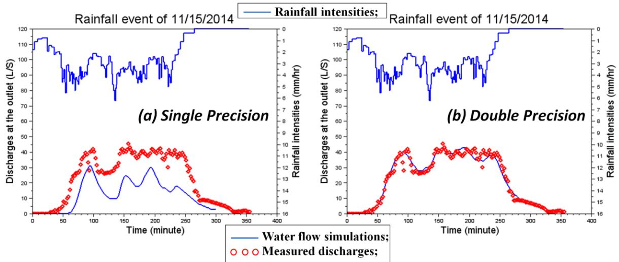
**Figure 8.** Change of the hydrograph due to the change from (a) single-precision to (b) double-precision floating-point format of the source code. The simulated discharges at the outlet (solid blue line) are compared with the measured data (red circles). Rainfall is plotted on the upper part.
