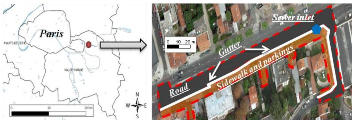
**Fig. 1** Study area at Eastern Paris, France. The catchment is delineated by red dashed lines, the sewer inlet is located at the northeast side of the catchment. In this picture, road area is marked as grey, gutter area is marked as white, sidewalk and parking areas are marked as brown.
