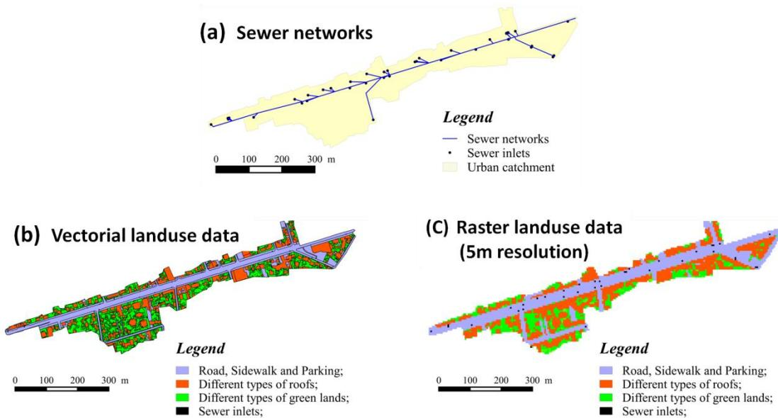
**Figure 5.** Input data for TRENNE: (a) Separate stormwater sewer networks, (b) Vectorial landuse data; (c) Raster landuse data with 5m resolution.
