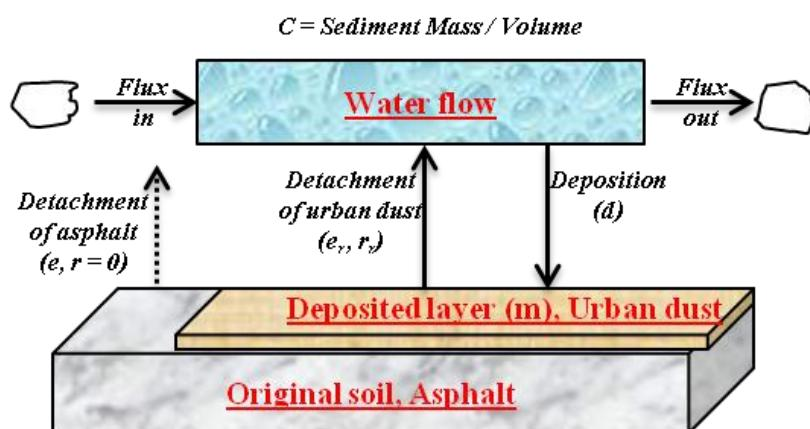
**Fig. 5** Concept of Hairsine - Rose Model.  $C$  represents the TSS concentration in mass per unit volume;  $m$  refers to the deposited sediment mass per unit area;  $e$  and  $r$  stand for the rate of rainfall-driven and flow-driven detachment for original soil, respectively;  $e_r$  and  $r_r$  mean respectively the rate of rainfall-driven and flow-driven detachment for the deposited layer; and  $d$  is the rate of TSS deposition from the water flow to the deposited layer.
