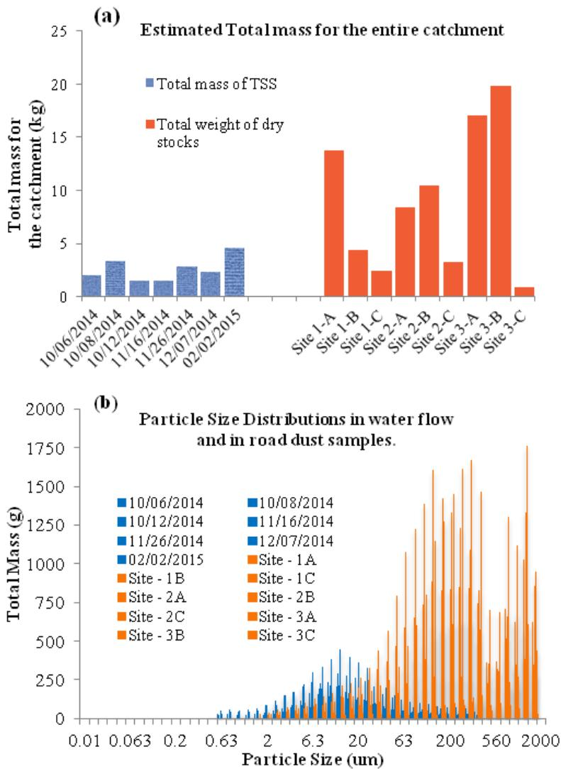
**Fig. 8** Measurements of Total Suspended Solids (TSS) and road dust in water flow and dry stock samples, respectively. For (a) Estimated total mass of TSS (blue bars) and road dust (orange bars) for different rainfall events and sampling sites, respectively. (b) Mass distributions of TSS (blue bars) and road dust (orange bars) for different rainfall events and sampling sites, respectively.
