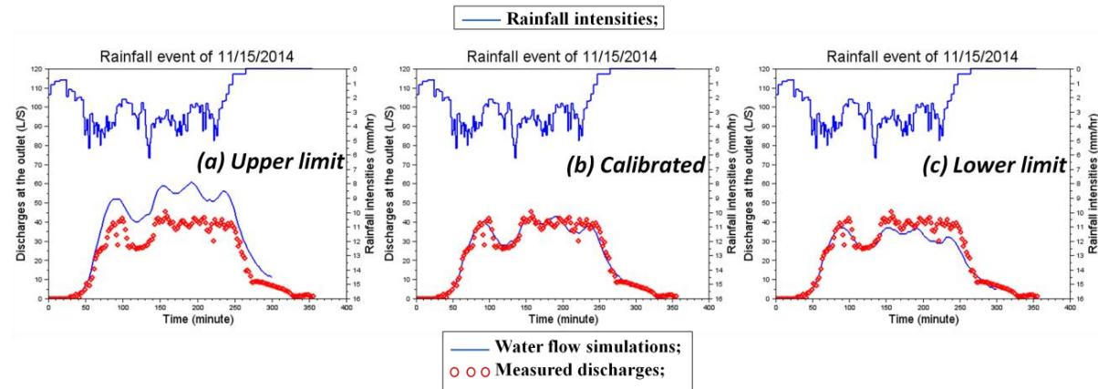
**Figure 9.** Hydrogram at the outlet of catchment using different values of water flow parameters. For (a) simulation using the upper limits of the parameter values; (b) simulation using the calibrated parameter values; (c) simulation using the lower limit of the parameter values. The simulated discharges at the outlet (solid blue line) are compared with the measured data (red circles). Rainfall is plotted on the upper part.
