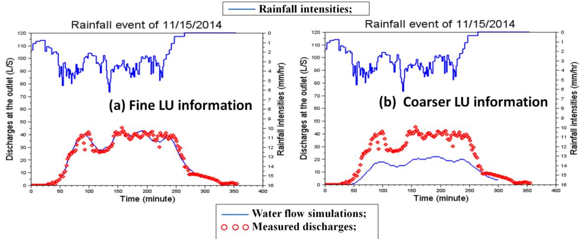
**Figure 11.** Hydrograph at the outlet of catchment using different landuse (LU) input maps. For (a) LU input map (5m) converted from fine LU information; (b) LU input map (5m) converted from coarser LU information. The simulated discharges at the outlet (solid blue line) are compared with the measured data (red circles). Rainfall is plotted on the upper part.
