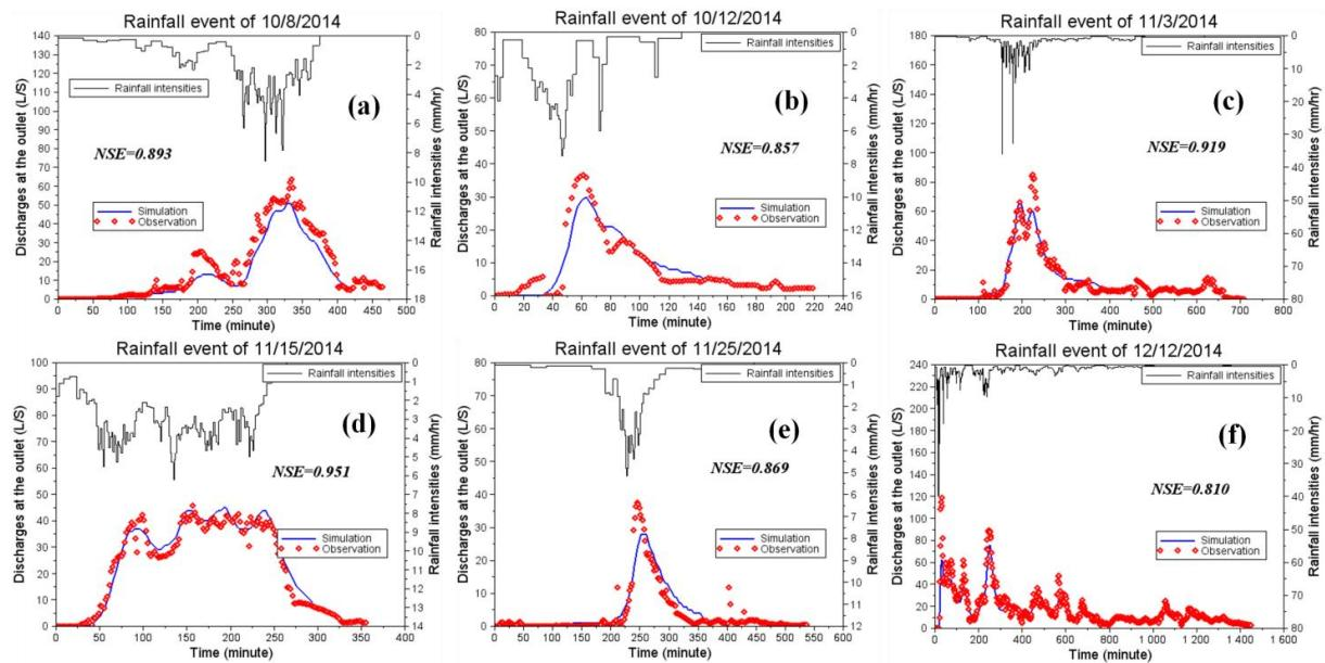
**Fig. 6** Water flow simulations using urban 2D/1D TRENNE model with the detailed DTM + LiDAR topography and Multi-sources Landuse. The simulated discharges at the network outlet (solid blue lines) are compared with the measured data (red circles). Rainfall is plotted on the upper part. For events (a) October 8, 2014;
