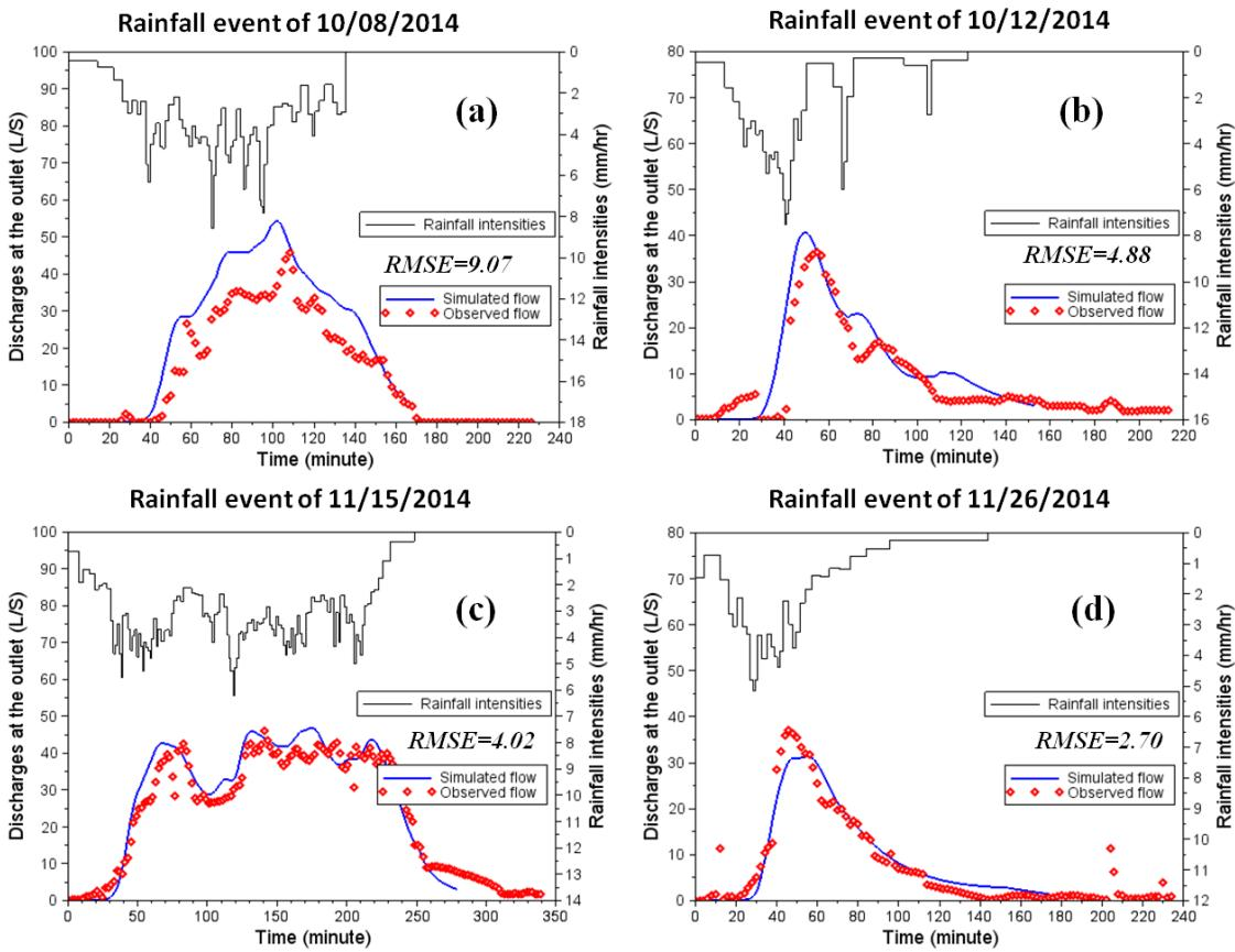
**Fig. 6** Water flow simulations using the integrated modelling approach. The simulated discharges at the network outlet (solid blue lines) are compared with the measured data (red circles). Rainfall is plotted on the upper part. For events (a) 8th of October 2014; (b) 12th of October 2014; (c) 15th of November 2014; (d) 26th of November 2014.
