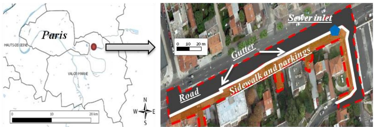
**Fig. 3** Study area in eastern Paris, France. The catchment is delineated by dashed red lines; the sewer inlet is located at the northeast side of the catchment. In this image, the road area is marked in grey, gutter area in white, and sidewalk and parking areas in brown.
