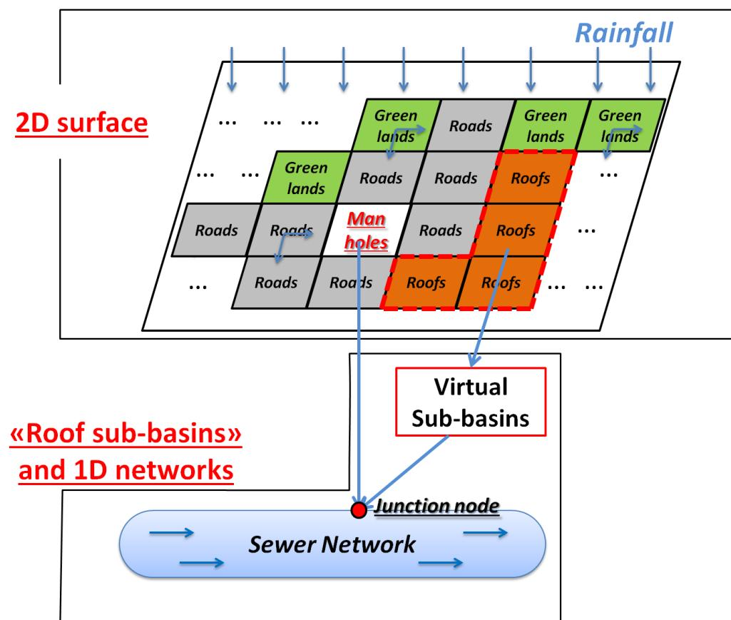
**Figure 1.** The scheme of the physically-based 2D/1D modelling platform TRENNE.
