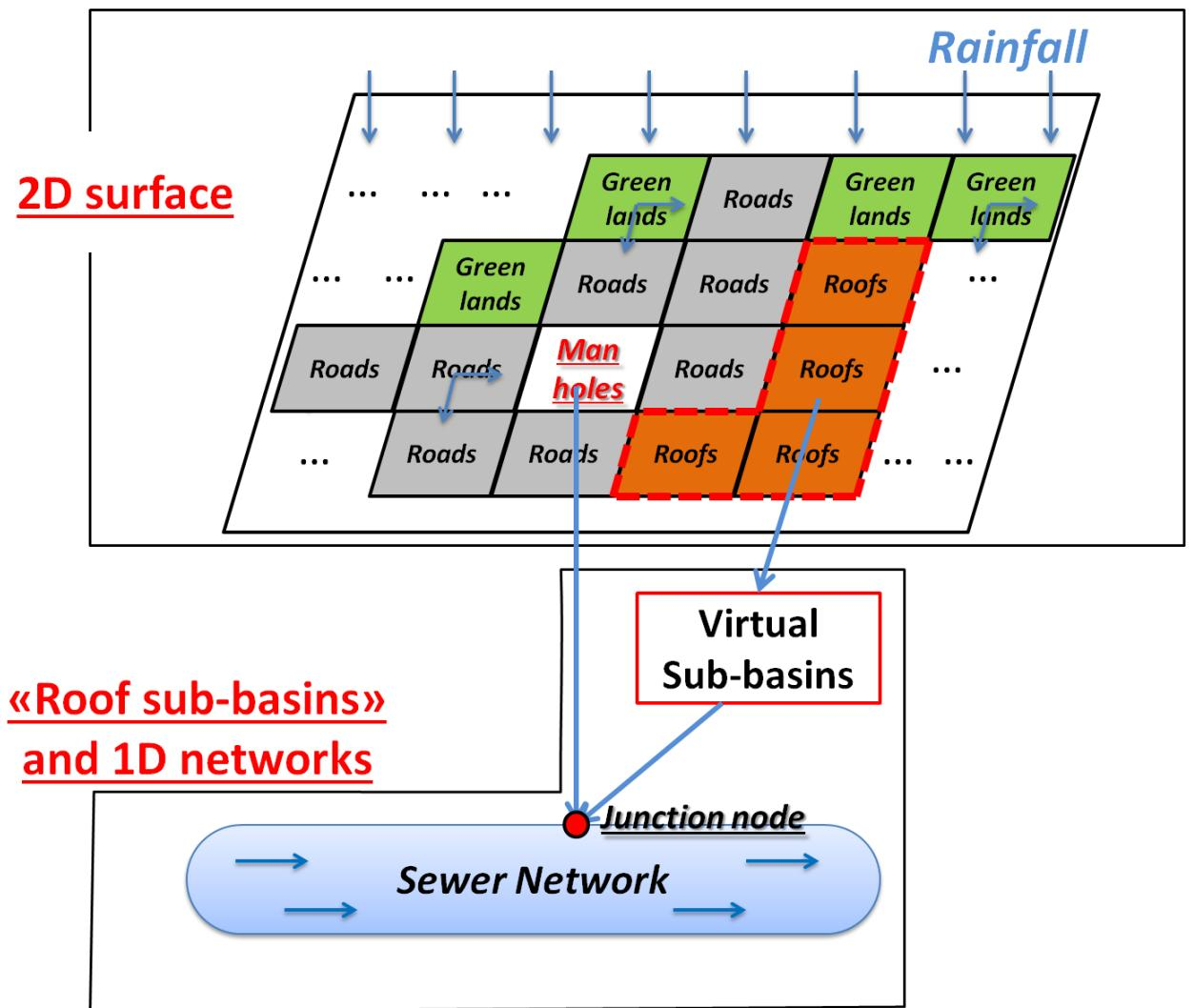
**Fig. 1.** The scheme of the 2D-surface and 1D-network modelling system TRENNE.
