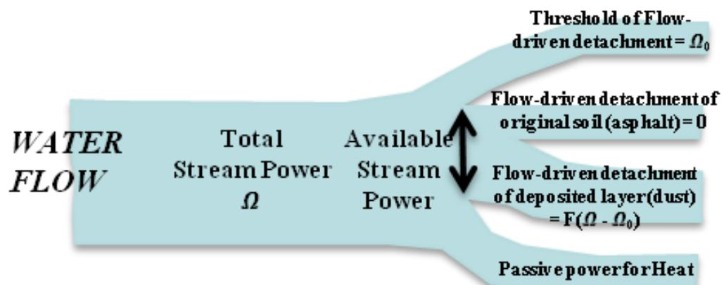
**Fig. 6** Flow diagram of the redistribution of Total Stream Power.
