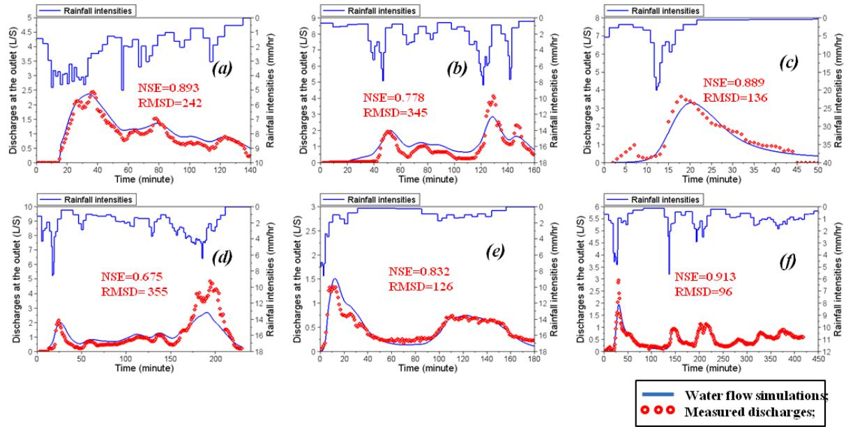
**Fig. 10** Water flow simulations using NSE and RMSD as objective functions. The simulated discharges at the outlet (solid blue line) are compared with the measured data (red circles). Rainfall is plotted on the upper part. For events (a) Feb. 28th 2015, (b) Oct. 6th 2014, (c) Oct. 7th 2014, (d) Nov. 14th 2014, (e) April. 2th 2015, (f) April. 3th 2015.
