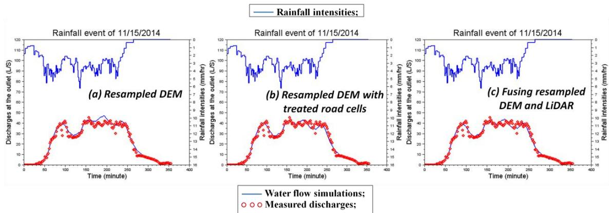
**Figure 10.** Hydrographs at the outlet of catchment using different topographic input maps. For (a) directly resampling the DEM data (25m) to 5m resolution; (b) resampling the DEM data (25m) to 5m resolution, and then lowering the identified road grid cells by 20cm; (c) resampling the road LiDAR data (20cm) and the DEM data
