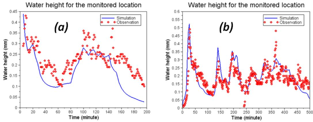
**Fig. 6** Spatial validation of the water depth simulation (solid blue line) using measured local water depth data (red circles) from the monitoring location inside the urban catchment (see Fig. 4b). For the events of: (a) April 2, 2015 and (b) April 3, 2015.
