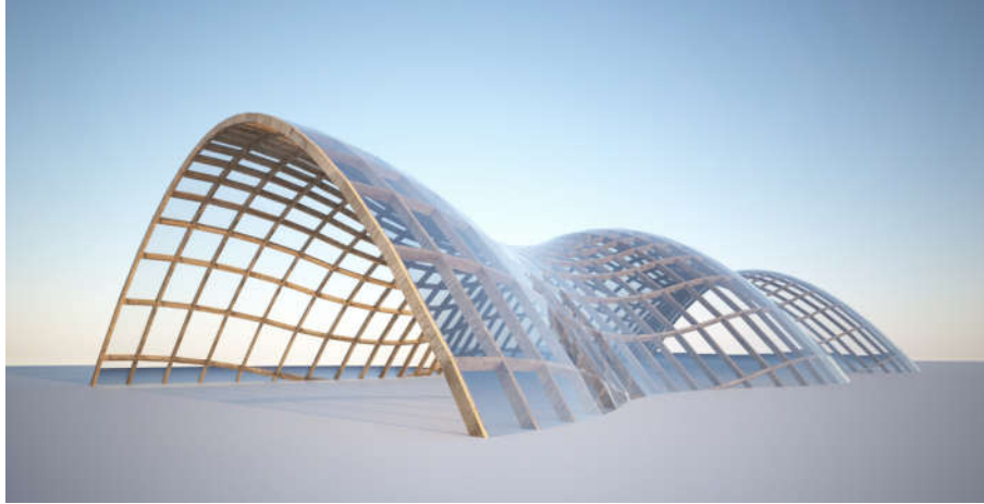
Figure 3.5 – Free-form generated as an isogonal moulding surface.
