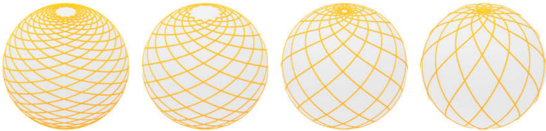
Figure 3.26 – Loxodromic parametrisations of a sphere: with \alpha = 20^\circ, 30^\circ, 45^\circ and 60^\circ from left to right
