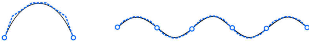
Figure 3.16 – Benchmark curves (continuous) with end points and inflection points, and the result of our algorithm (dashed lines).
