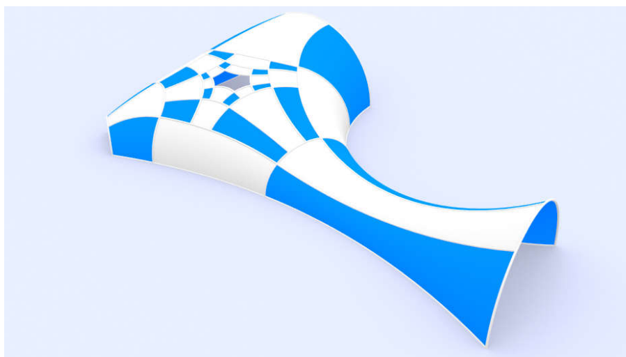
Figure 4.31 – Hole-filling strategy applied iteratively three times on a non-regular hole.
