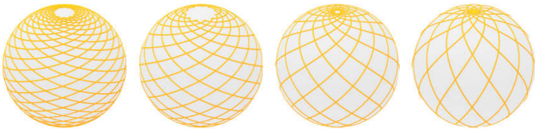
Figure 3.26 – Loxodromic parametrisations of a sphere: with \alpha = 20^\circ, 30^\circ, 45^\circ and 60^\circ from left to right
