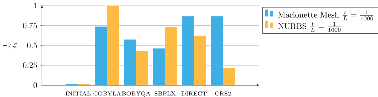
Figure 6.22 – Optimal values found for the minimisation of displacement under self-weight ( \frac{t}{L} = \frac{1}{1000} ).
