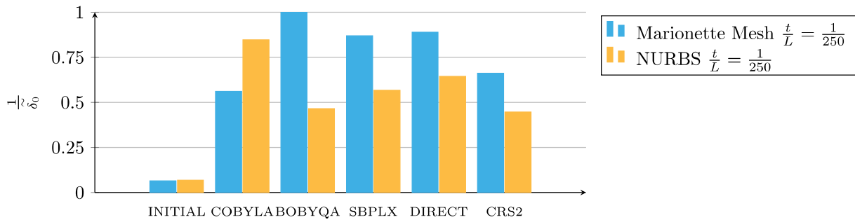
Figure 6.25 – Optimal values found for the minimisation of displacement under self-weight ( t/L = 1/250 ).
