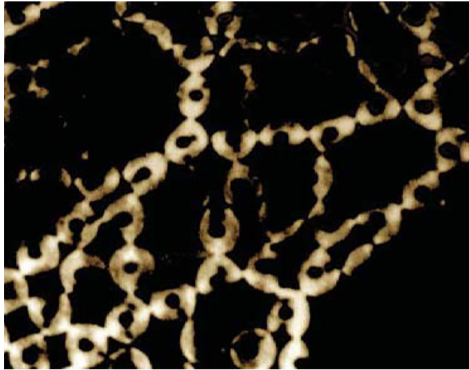
Figure 1.2: Photoelastic image of a small assembly of disks (from Dantu [57]).
