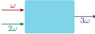
Figure 1.7: Scheme of frequency tripling realized through SFG.
