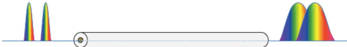
Figure 1.12: Inter-symbol interference due to chromatic dispersion
