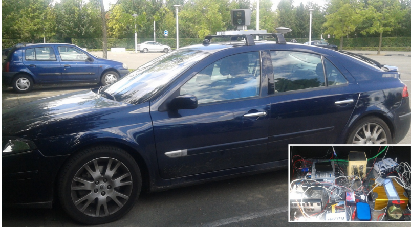
Figure 4-1: Test Vehicle used for vehicle tracking experiment. Lidar and GPS are mounted on top of the vehicle and embedded computers are located in the trunk of the vehicle (see picture inset).
