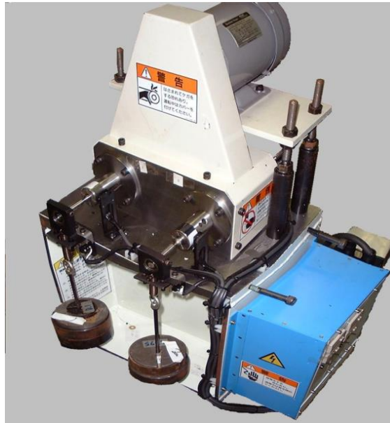
Figure 1-12 Dual-spindle rotating bending fatigue testing machine [61].
