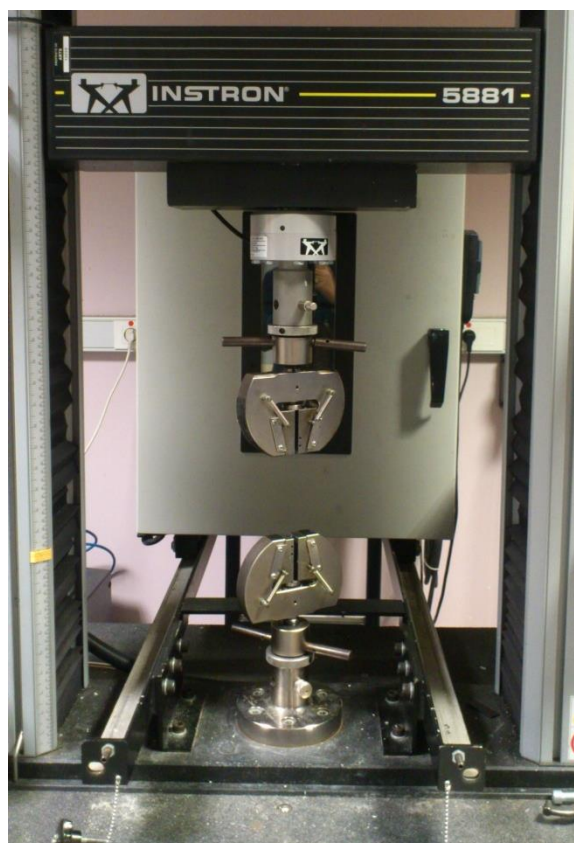
Figure 2-18 Uniaxial tensile test set-up.
