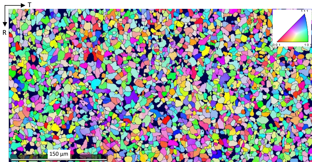
Figure 2-6 Inverse pole figure about the normal direction (martensite grains are represented in black).
