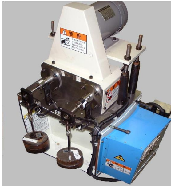
Figure 1-12 Dual-spindle rotating bending fatigue testing machine [61].
