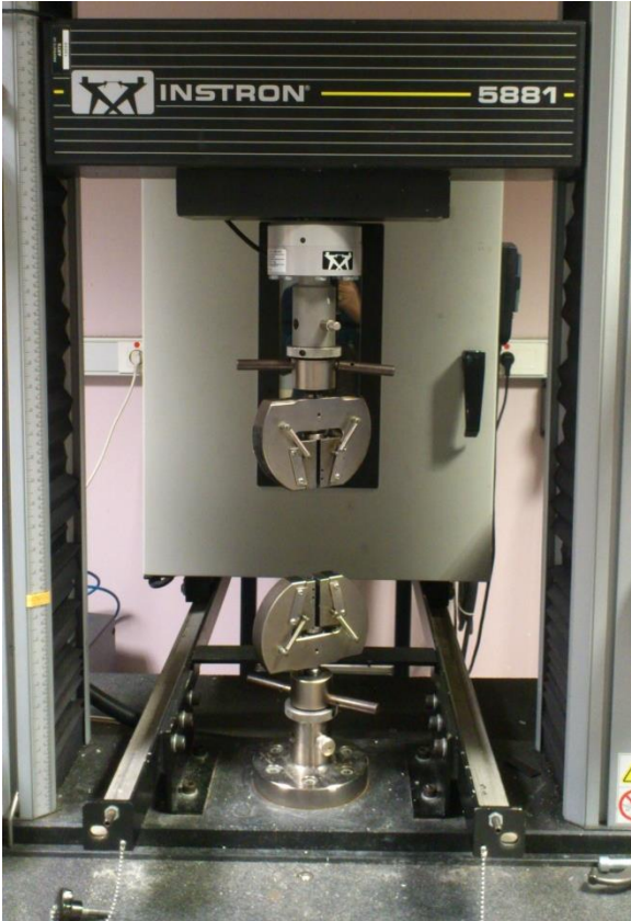
Figure 2-18 Uniaxial tensile test set-up.
