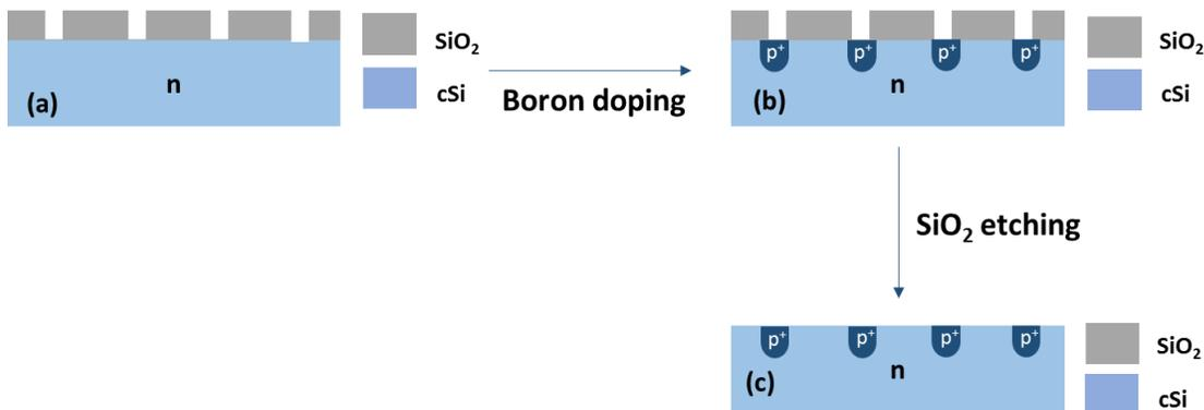
Fig.5.1: Schematic diagram of local doping fabrication process. (a) Forming holes in SiO<sub>2</sub> using approach B (ch.4), (b) Boron doping by thermal diffusion or ion implantation, and (c) SiO<sub>2</sub> etching.
