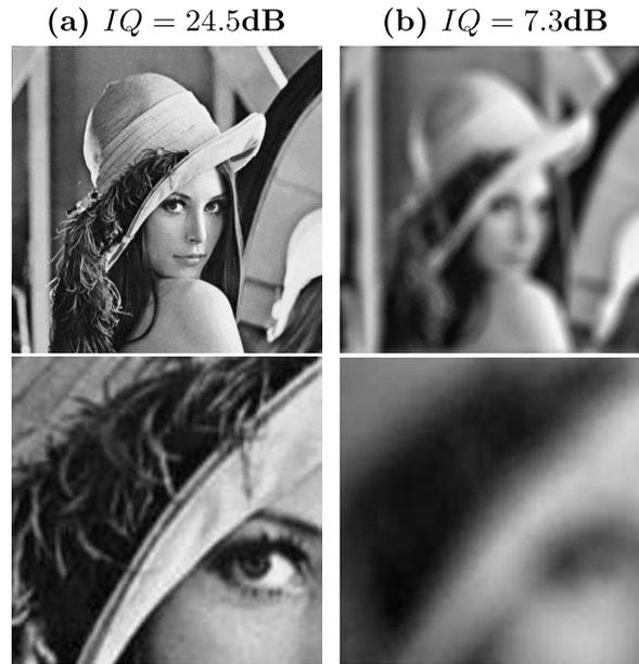
FIGURE 2.15: Images produced by a diffraction limited system with  $SNR = 34dB$  after deconvolution at (a)  $\psi = 0\lambda$  and (b)  $\psi = 2.0\lambda$ .
