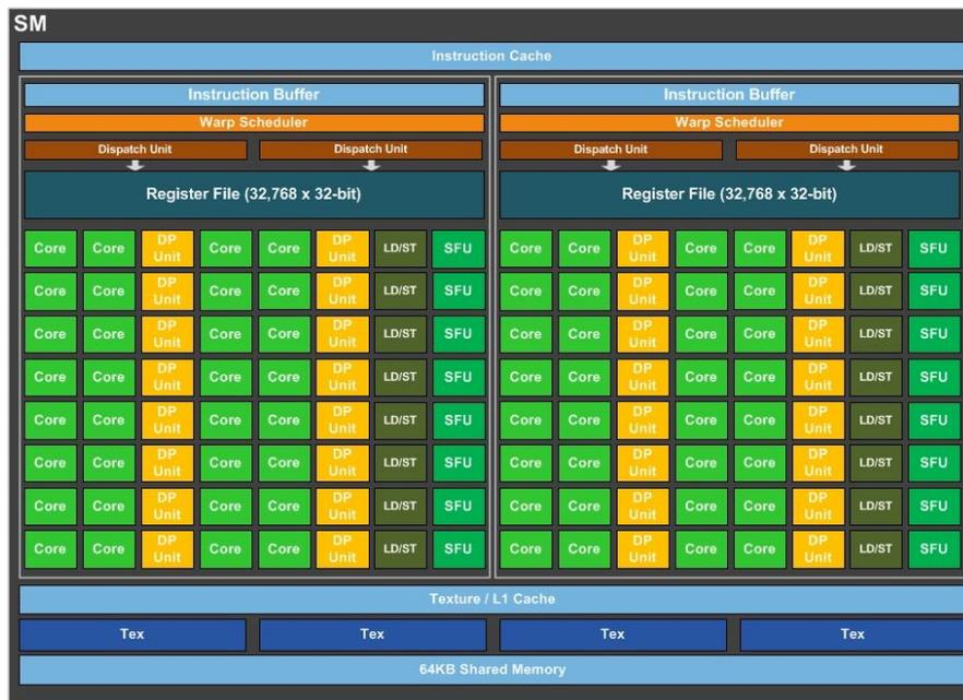
FIGURE 2.9: Tesla P100 streaming multiprocessor [46].
