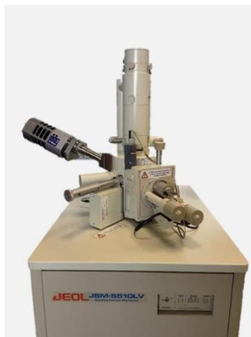
**Figure II.14 : MEB JEOL JSM-5510**
