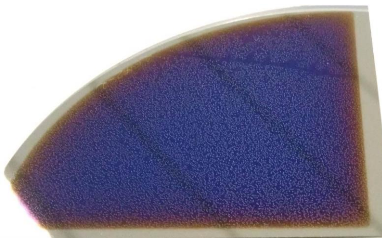
Figure 3.14: \text{Al}_2\text{O}_3/\text{a-SiN}_x\text{:H} passivated sample presenting blistering.
