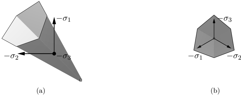
Figure 4.3: Mohr-Coulomb yield surface (a) in the (-\sigma_1, -\sigma_2) plane, (b) from the principal stress space diagonal.
