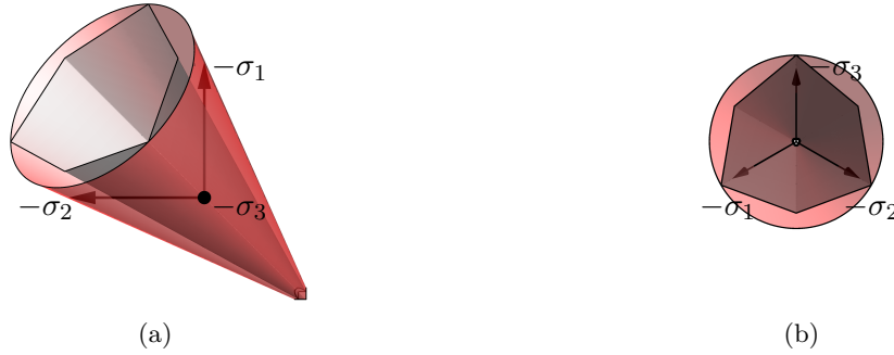
Figure 4.4: Drucker-Prager conic yield surface circumscribing the Mohr-Coulomb pyramidal yield surface (a) in the (-\sigma_1, -\sigma_2) plane, (b) from the principal stress space diagonal.
