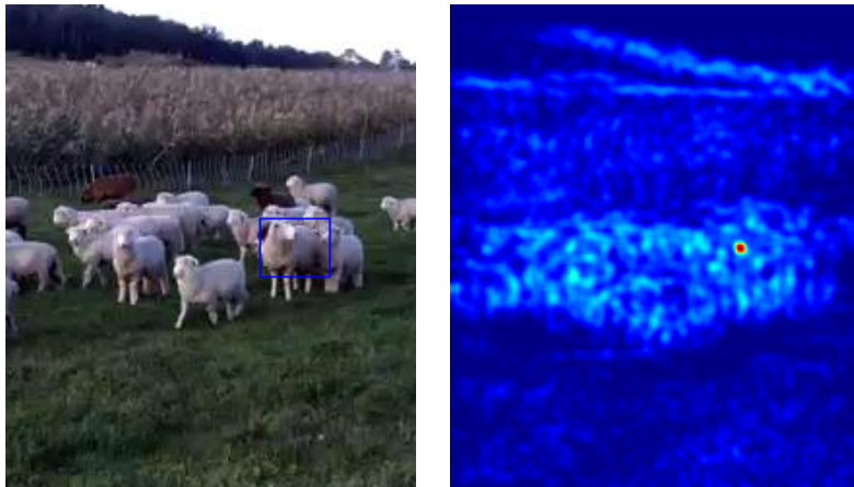
FIGURE 2.22: GHT on a scene, with the squared sheep used as a model
