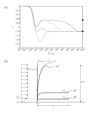
Figure 2.5: Reconfiguration in a Blasius boundary layer, anchorage point  $x_0 = 10^7$ . (a) Vogel exponent  $\nu$  as a function of the Cauchy number  $C_{Y,uni}$ ,  $L_B = 10^{-3}$  (——),  $L_B = 10^{-2}$  (···),  $L_B = 10^{-1}$  (——),  $L_B = 1$  (—·—). Asymptotic Vogel exponent predicted by equation (2.23), uniform flow profile ( $\circ$ ), linear flow profile ( $\Box$ ). (b) Zoom near the clamped edge of a beam bending in a Blasius boundary layer,  $L_B = 10^{-2}$ .
