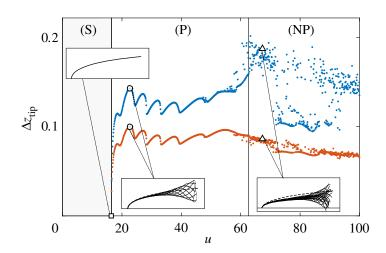
**Figure 4.** Vertical amplitude of flapping at the tip (blue) and standard deviation (orange) versus the reduced velocity u, for  $\beta = 0.5$ ,  $\lambda = 10$ . Examples of deformation modes are shown in the thumbnails for u = 16.4 (square, static regime (S)), u = 22.7 (circle, periodic regime (P)) and u = 67.3 (triangle, non-periodic regime (NP)). Static equilibrium shape superimposed (dashed lines).
