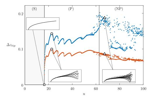
Figure 4.4: Vertical amplitude of flapping at the tip (blue) and standard deviation (orange) versus the reduced velocity u, for  $\beta = 0.5$ ,  $\lambda = 10$ . Static regime (S), periodic regime (P) and non-periodic regime (NP). Examples of deformation modes are shown in the thumbnails for u = 16.4 ( $\Box$ , static regime), u = 22.7 (o, periodic regime), u = 67.3 ( $\Delta$ , non-periodic regime). Static equilibrium shape superimposed (--).
