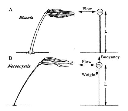
Figure 1.12: Examples of models used in the numerical work of Mark Denny: A. cantilever beam model with lumped mass at the top, for the modelling of the bending deformation of the stipitate kelp *Eisenia arboarea*. B. Spring-chain model with lumped mass at the top, for the modelling of the tensile deformation of *Nereocystis luetkeana*, from Denny et al. (1998).
