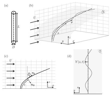
Figure 1: (a) Dimensions of the undeformed cylinder and centerline (broken line). (b) 3D view of the centerline of the vibrating cylinder, static deflection  $r_0(s)$  (broken black line), fully deformed shape r(s,t) (solid grey line). The  $\pi$ -plane in grey indicates the surface upon which the vibration occurs. (c) Projection of the deformation on the plane of static deflection (xz-plane). (d) Projection of the deformation on the surface of vibration ( $\pi$ -surface or sy-surface).
