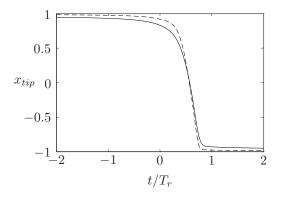
Figure 3.7: Horizontal displacement of the tip during flow reversal against the rescaled time  $t/T_r$ , for  $\alpha = 10^2$ ,  $T_r = 0.2$  ( $\omega = 1$ ) and  $\lambda = 12.7$  (---),  $\lambda = 127$  (---).
