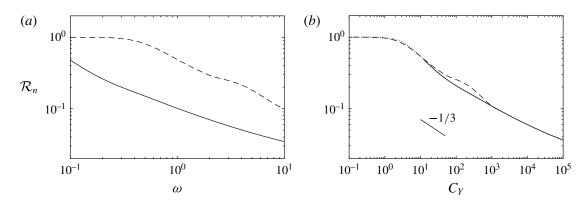
FIGURE 11. Shear reconfiguration number in the large-amplitude regime for  $\lambda = 12.7$ , against (*a*) the frequency ratio  $\omega$ , (*b*) the Cauchy number  $C_Y$ , for  $\alpha = 10^0$  (---),  $\alpha = 10^1$  (---). Static solution obtained with (5.6) (...., on (*b*) only).
