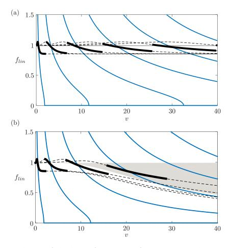
Figure 5.5: Evolution of the linear frequencies of the coupled wake-structure system with the reduced velocity v, for (a) the straight case and (b) the deflected case  $\Lambda = 10^3$ . The unconditionally unstable free wake spectrum is represented by the grey area. The structural modes in blue are always stable. The coupled modes, displayed in black, are always unstable. The most unstable mode for a given range of v is emphasized in bold.
