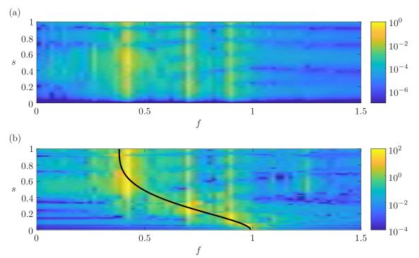
Figure 6: Spanwise distribution of power spectral density of (a) the structural motion Y and (b) the wake oscillator q, for  $\Lambda = 10^3$  and u = 49.0. The natural shedding frequency  $f_w^0(s)$  given by the Strouhal law is superimposed in (b) (---).
