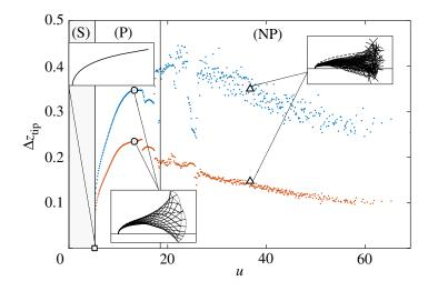
**Figure 6.** Vertical amplitude of flapping at the tip (blue) and standard deviation (orange) versus the reduced velocity *u*, for  $\beta = 0.1$ ,  $\lambda = 10$ . Examples of deformation modes are shown in the thumbnails for u = 5.2 (square, static regime (S)), u = 13.2 (circle, periodic regime (P)) and u = 36.7 (triangle, non-periodic regime (NP)). Static equilibrium shape superimposed (dashed lines).
