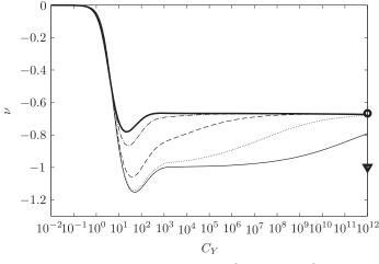
**Fig. 8.** Vogel exponent  $\nu$  of a tapered beam for increasing Cauchy numbers  $C_{Y}$ ,  $\delta = 10^{-3}$  (----),  $\delta = 10^{-2}$  (·-·-),  $\delta = 10^{-1}$  (----),  $\delta = 1$  (----), and  $\delta = +\infty$  (thick ----). Asymptotic Vogel exponent predicted by Eq. (23), constant width ( $\circ$ ) and linear width ( $\nabla$ ).
