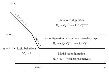
FIGURE 12. Schematic view of the reconfiguration regimes in the amplitude–frequency space.
