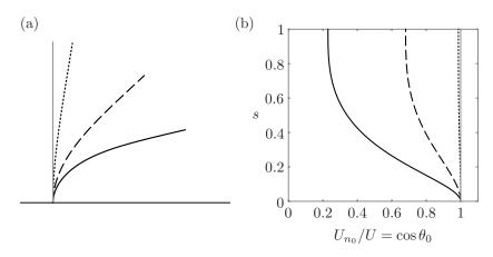
Figure 5.2: (a) Deflection in the xz-plane and (b) normal velocity profile normalized by the horizontal velocity, in the straight case (grey —), and in deflected cases  $C_Y = 10^0$  ( $\cdots$ ),  $C_Y = 10^1$  (--), and  $C_Y = 10^2$  (black —) for  $\Lambda = 10^3$ .
