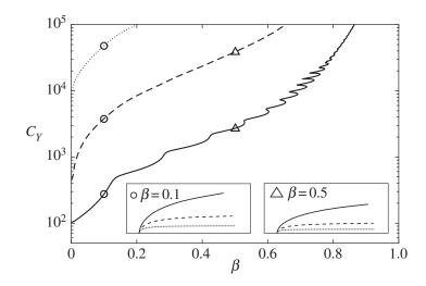
**Figure 3.** Critical Cauchy number  $C_{Y,c}$  as a function of the mass ratio  $\beta$  and static equilibrium shape at the stability threshold for two specific values of the mass ratio, for  $\lambda = 10$  (solid line),  $\lambda = 10^2$  (dashed line) and  $\lambda = 10^3$  (dotted line).
