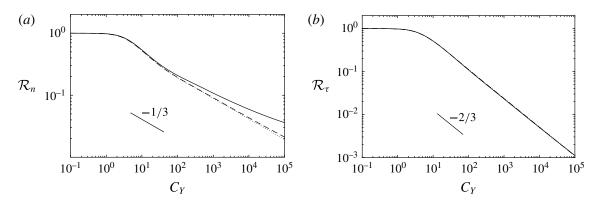
FIGURE 14. Variations of the static reconfiguration numbers obtained with (5.6) ((*a*) shear, (*b*) tensile) as a function of the Cauchy number  $C_Y$ , for  $\lambda = 12.7$  (---),  $\lambda = 1270$  (---),  $\lambda = 1270$  (---).
