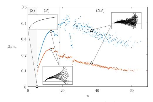
Figure 4.6: Vertical amplitude of flapping at the tip (blue) and standard deviation (orange) versus the reduced velocity u, for  $\beta = 0.1$ ,  $\lambda = 10$ . Static regime (S), periodic regime (P) and non-periodic regime (NP). Examples of deformation modes are shown in the thumbnails for u = 5.2 ( $\Box$ , static regime), u = 13.2 ( $\circ$ , periodic regime), u = 36.7 ( $\Delta$ , non-periodic regime). Static equilibrium shape superimposed (--).
