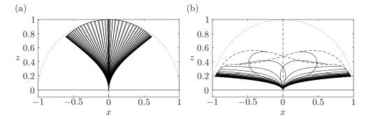
Figure 3.6: Snapshots of the deforming structure over one cycle (—) and tip trajectory (---) obtained with Eq. (3.8) for  $\lambda = 12.7$ ,  $\alpha = 10^2$ . (a)  $\omega = 10^{-2}$ , (b)  $\omega = 1$ .
