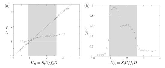
Figure 1.11: Lock-in of a flexibly mounted, rigid circular cylinder, from Khalak and Williamson (1997). Evolution of (a) the frequency f of the VIVs normalized by the natural frequency  $f_s$  of the solid oscillator, and (b) the amplitude of vibrations Y normalized by the diameter of the cylinder D, as functions of the reduced velocity  $U_R = S_t U/f_s D$ . The grey zone corresponds to lock-in.
