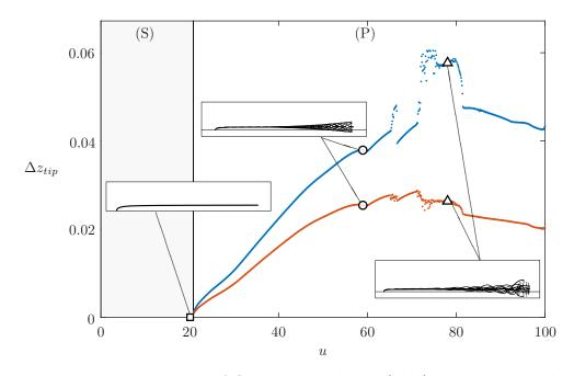
Figure 4.5: Vertical amplitude of flapping at the tip (blue) and standard deviation (orange) versus the reduced velocity u, for  $\beta = 0.5$ ,  $\lambda = 10^3$ . Static regime (S) and periodic regime (P). Examples of deformation modes are shown in the thumbnails for u = 20.0 ( $\Box$ , static regime), u = 59.0 (o, periodic regime), u = 78.0 ( $\Delta$ , periodic regime as well). Static equilibrium shape superimposed (--).
