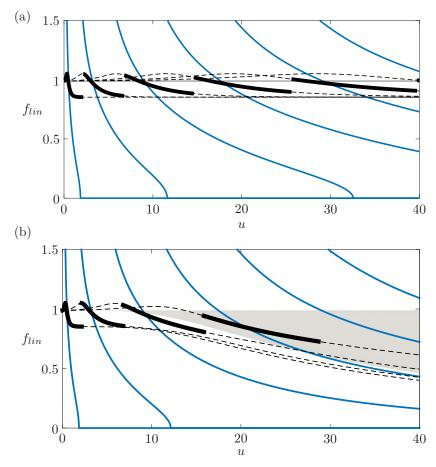
Figure 5: Evolution of the linear frequencies of the coupled wake-structure system with the reduced velocity u, for (a) the straight case and (b) the deflected case  $\Lambda = 10^3$ . The unconditionally unstable free wake spectrum is represented by the grey area. The structural modes in blue are always stable. The coupled modes, displayed in black, are always unstable. The most unstable mode for a given range of u is emphasized in bold.
