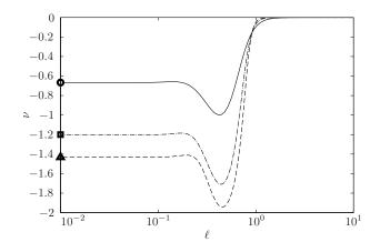
Figure 2.3: A uniform beam in a shear flow. Variation of the Vogel exponent in the  $\ell - \nu$  space, uniform flow profile  $\mu/2 = 0$  (----), linear flow profile  $\mu/2 = 1$  (---), quadratic flow profile  $\mu/2 = 2$  (---). Asymptotic Vogel exponent predicted by equation (2.23), uniform flow profile  $\mu/2 = 0$  ( $\circ$ ), linear flow profile  $\mu/2 = 1$  ( $\Box$ ), quadratic flow profile  $\mu/2 = 2$  ( $\Delta$ ).
