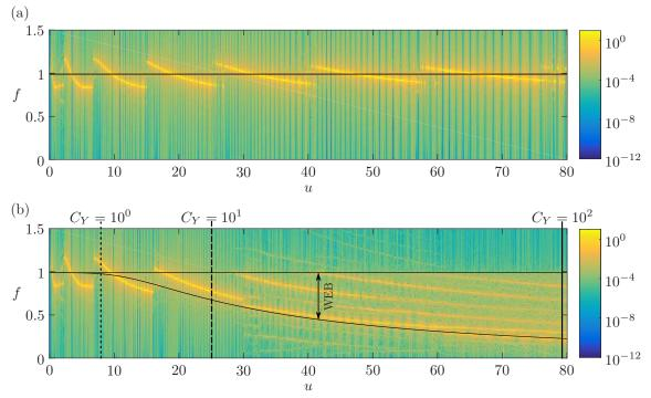
Figure 3: Comparison between the power spectral densities of the motion at the tip Y(s = 1, t) in (a) the straight case and (b) the deflected case  $\Lambda = 10^3$ , for varying reduced velocities u. The natural wake excitation bandwidth (WEB) is superimposed. The particular values of the reduced velocity u corresponding to Fig. 2 are indicated as well.
