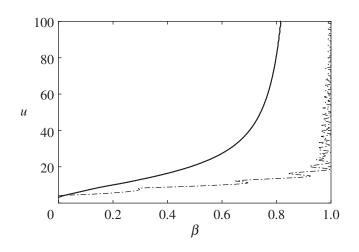
**Figure 11.** Linear stability thresholds obtained with the full equation (3.6) for  $\lambda = 10^3$  (dotted line), with the equation relative to the axial configuration (3.7) (dashed dotted line) and with the asymptotic equation (B 1) for  $\lambda = 10^3$  (solid line).
