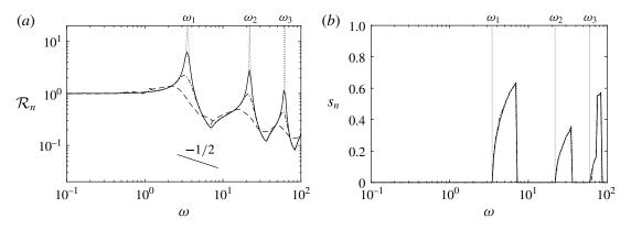
FIGURE 9. Shear reconfiguration number (*a*) and location of maximum shear stress along the span (*b*), in the modal regime, against the frequency ratio, for  $K_C = 10^{-2}$  (----),  $K_C = 10^{-1}$  (----),  $K_C = 10^0$  (----) and analytical solution for  $K_C \rightarrow 0$  (·····-).
