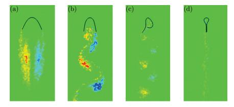
Figure 1.9: Bending modes found by Yang and Liu (2016): (a) stable U-shaped mode, (b) slight swing, (c) violent flapping, (d) closed mode.
