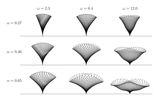
Figure 3.3: Phase-averaged experimental oscillation cycle for varying amplitudes  $\alpha$  and frequencies  $\omega$ . Snapshots of the structural shape (—) and tip trajectory (—).
