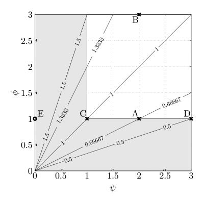
Figure 2.8: Absolute value of the Vogel exponent in the reduced parameter space  $\psi - \phi$ . The domain shaded in grey corresponds to non-physical ranges. Practical cases: A,B,C,D,E (see text for the details).
