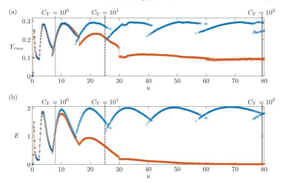
Figure 7: Comparison of (a) the RMS amplitude of vibration  $Y_{rms}$  and (b) the total energy transfer E from the wake to the structure, between the straight case (blue  $\circ$ ) and the deflected case  $\Lambda = 10^3$  (orange  $\bigtriangledown$ ) for varying reduced velocities u. The particular values of the reduced velocity u corresponding to Fig. 2 are indicated as well.
