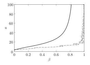
Figure E.1: Linear stability thresholds obtained with the full equation (4.10) for  $\lambda = 10^3$  (· · · ), with the equation relative to the axial configuration (4.11) (- · -), and with the asymptotic equation (E.1) for  $\lambda = 10^3$  (----).
