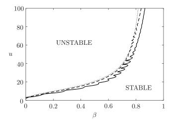
Figure 4.2: Critical velocity  $u_c$  as a function of the mass ratio  $\beta$ , for  $\lambda = 10$  (----),  $\lambda = 10^3$  (· · · ).
