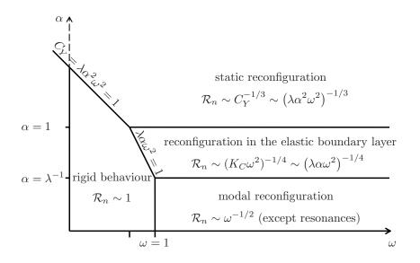
Figure 3.12: Schematic view of the reconfiguration regimes in the amplitude-frequency space.
