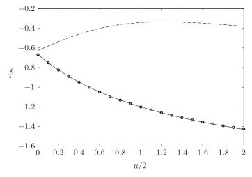
**Fig. 10.** Asymptotic Vogel exponent  $\nu_{\infty}$  for large Cauchy numbers as a function of the flow profile exponent  $\mu/2$ . Henriquez and Barrero-Gil, 2014 (---), present results given by Eq. (23) (\_\_\_\_\_), and numerical simulations at  $C_{\rm Y} = 10^5$  (o).
