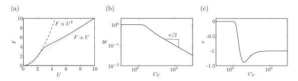
Figure 1.6: Schematic view of the loading-drag relationship in the different parameter spaces (arbitrary units). U: reference flow velocity, F: drag force,  $C_Y$ : Cauchy number,  $\mathcal{R}$ : reconfiguration number, and  $\nu$ : Vogel exponent.
