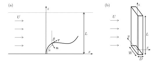
Figure 3.1: (a) Side view of the bending structure. (b) Dimensions of the undeformed blade.
