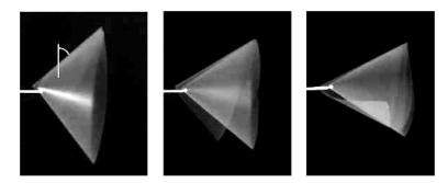
Figure 1.7: Experimental setup of Schouveiler and Boudaoud (2006): a circular plastic sheet cut along a radius rolls up into a cone as the flow velocity (from left to right) is increased, from left to right.
