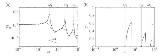
Figure 3.9: Shear reconfiguration number (a) and location of maximum shear stress along the span (b), in the modal regime, against the frequency ratio, for  $K_C = 10^{-2}$ (---),  $K_C = 10^{-1}$  (-·-),  $K_C = 10^0$  (- - -), and analytical solution for  $K_C \to 0$ (····).
