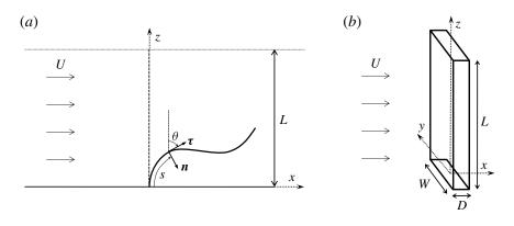
FIGURE 1. (a) Side view of the bending structure. (b) Dimensions of the undeformed blade.
