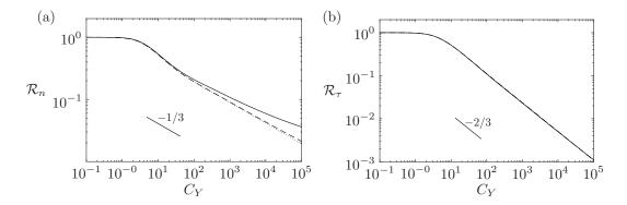
Figure D.1: Variations of the static reconfiguration numbers obtained with Eq. 3.21 ((a) shear, (b) tensile) as a function of the Cauchy number  $C_Y$ , for  $\lambda = 12.7$  (---),  $\lambda = 1270$  (····).
