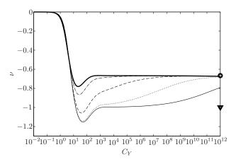
Figure 2.7: Vogel exponent  $\nu$  of a tapered beam for increasing Cauchy numbers  $C_Y$ ,  $\delta = 10^{-3}$  (----),  $\delta = 10^{-2}$  (···),  $\delta = 10^{-1}$  (---),  $\delta = 1$  (-·-),  $\delta = +\infty$  (thick ----). Asymptotic Vogel exponent predicted by equation (2.23), constant width ( $\circ$ ), linear width ( $\nabla$ ).
