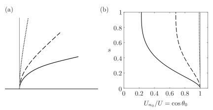
Figure 2: (a) Deflection in the xz-plane and (b) normal velocity profile normalized by the horizontal velocity, in the straight case (grey —), and in deflected cases  $C_Y = 10^0$  (· · ·),  $C_Y = 10^1$  (- - -), and  $C_Y = 10^2$  (black —) for  $\Lambda = 10^3$ .
