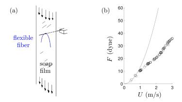
Figure 1.4: (a) Experimental setup of Alben et al. (2004) and (b) evolution of the drag force on the flexible fibre as a function of the velocity of the soap film.
