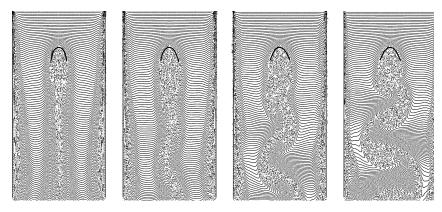
Figure 1.8: Flow past a flexible fibre at varying Reynolds number (a)  $R_e = 82.5$ , (a)  $R_e = 165$ , (a)  $R_e = 330$  (a)  $R_e = 660$ , for a fixed Cauchy number, from Zhu (2007).
