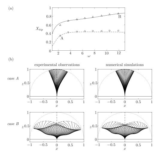
Figure 3.4: Comparison between experimental observations and numerical simulations. (a) Amplitude of the deflection at the tip against the frequency ratio, for  $\alpha = 0.27$  (numerical -, experimental  $\circ$ ),  $\alpha = 0.65$  (numerical -, experimental  $\triangle$ ). (b) Deformed shape found experimentally (left) and numerically (right), in case A (top,  $\alpha = 0.27$ ,  $\omega = 2.3$ ) and case B (bottom,  $\alpha = 0.65$ ,  $\omega = 12.0$ ).
