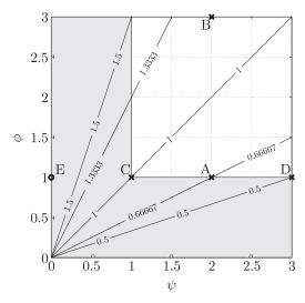
**Fig. 9.** Absolute value of the Vogel exponent in the reduced parameter space  $\psi - \phi$ . The domain shaded in grey corresponds to non-physical ranges. Practical cases: A–E (see text for the details).
