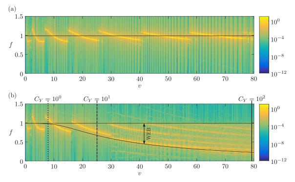
Figure 5.3: Comparison between the power spectral densities of the motion at the tip Y(s = 1, t) in (a) the straight case and (b) the deflected case  $\Lambda = 10^3$ , for varying reduced velocities v. The natural wake excitation bandwidth (WEB) is superimposed. The particular values of the reduced velocity v corresponding to Fig. 5.2 are indicated as well.
