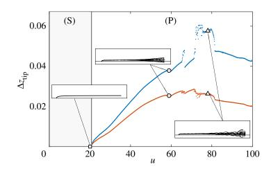
**Figure 5.** Vertical amplitude of flapping at the tip (blue) and standard deviation (orange) versus the reduced velocity u, for  $\beta = 0.5$ ,  $\lambda = 10^3$ . Examples of deformation modes are shown in the thumbnails for u = 20.0 (square, static regime (S)), u = 59.0 (circle, periodic regime (P)) and u = 78.0 (triangle, periodic regime also). Static equilibrium shape superimposed (dashed lines).
