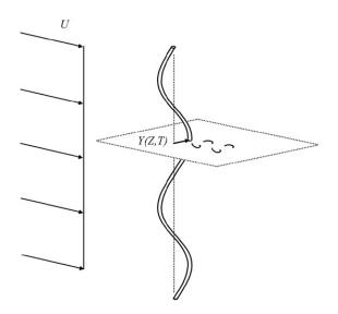
Figure 1.10: Vortex-induced vibration of a cable in transverse flow, from Violette et al. (2010). The wake vortices alternatively shed in the plane of the cross-sections force the structure into transverse oscillations.
