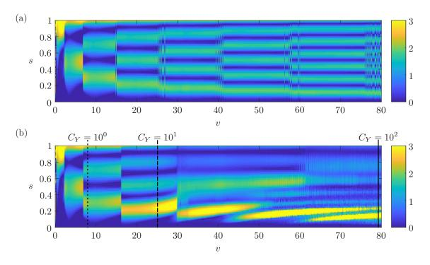
Figure 5.8: Comparison of the spanwise distributions of energy transfer from the wake to the structure between (a) the straight case and (b) the deflected case  $\Lambda = 10^3$ , for varying reduced velocities v. The colorplots show the mean work of the oscillating lift force  $\langle e \rangle$  normalized by the total energy transfer E. The particular values of the reduced velocity v corresponding to Fig. 5.2 are indicated as well.
