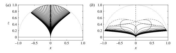
FIGURE 6. Snapshots of the deforming structure over one cycle (——) and tip trajectory (---) obtained with (2.8) for  $\lambda = 12.7$ ,  $\alpha = 10^2$ . (a)  $\omega = 10^{-2}$ , (b)  $\omega = 1$ .
