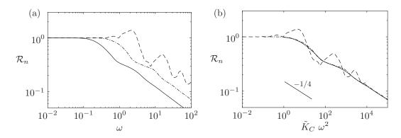
Figure 3.10: Shear reconfiguration number in the convective regime against (a) the frequency ratio  $\omega$ , (b) the rescaled parameter  $K_C \omega^2$ , for  $K_C = 10^0 (---)$ ,  $K_C = 10^1 (---)$ ,  $K_C = 10^2 (---)$ .
