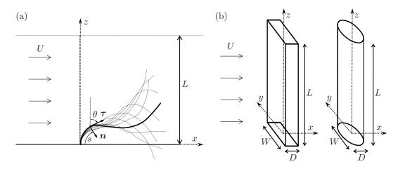
Figure 4.1: (a) Side view of the deforming structure. (b) Examples of geometries of two undeformed structures with different cross-section shapes.
