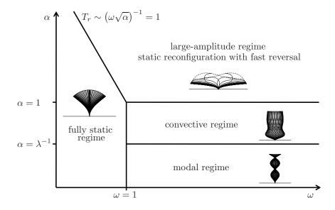
Figure 3.8: Schematic view of the kinematic regimes in the amplitude-frequency space.
