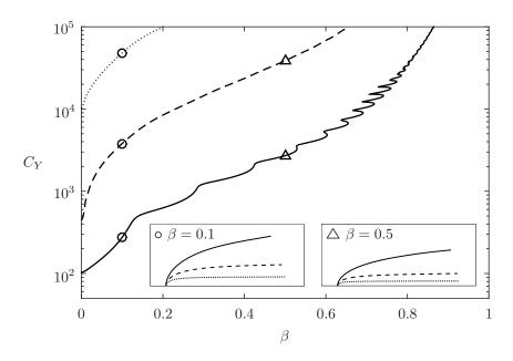
Figure 4.3: Critical Cauchy number  $C_{Y,c}$  as a function of the mass ratio  $\beta$  and static equilibrium shape at the stability threshold for two specific values of the mass ratio, for  $\lambda = 10$  (----),  $\lambda = 10^3$  (···).
