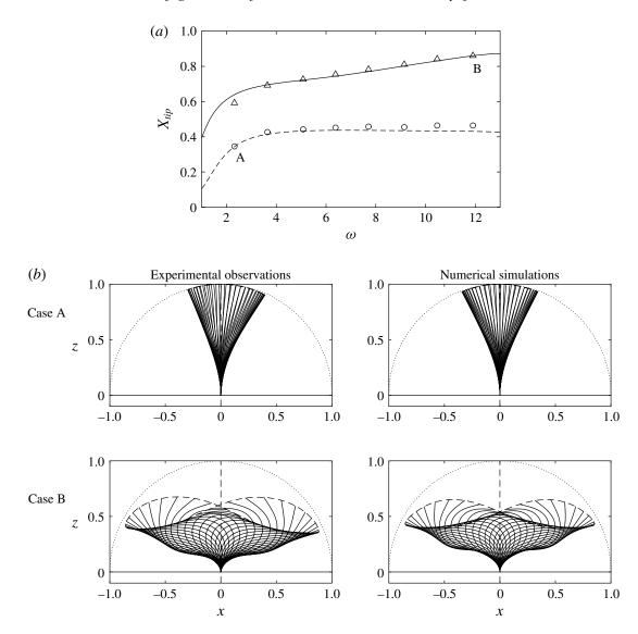
FIGURE 4. Comparison between experimental observations and numerical simulations. (a) Amplitude of the deflection at the tip against the frequency ratio, for  $\alpha = 0.27$  (numerical --, experimental  $\bigcirc$ ),  $\alpha = 0.65$  (numerical --, experimental  $\triangle$ ). (b) Deformed shape found experimentally (left) and numerically (right), in case A (top,  $\alpha = 0.27$ ,  $\omega = 2.3$ ) and case B (bottom,  $\alpha = 0.65$ ,  $\omega = 12.0$ ).
