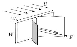
Figure 1.5: Experimental setup of Gosselin et al. (2010): a rectangular plate is clamped in the middle in a transverse flow of velocity U.
