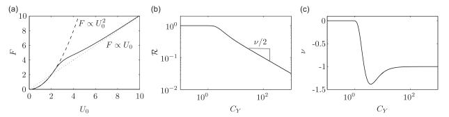
**Fig. 2.** Schematic view of the loading-drag relationship in the different parameter spaces (arbitrary units).  $U_0$ : reference flow velocity, F: drag force,  $C_Y$ : Cauchy number,  $\mathcal{R}$ : Reconfiguration number, and  $\nu$ : Vogel exponent.
