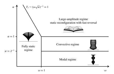
FIGURE 8. Schematic view of the kinematic regimes in the amplitude-frequency space.
