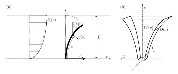
Figure 2.1: Description of the system. (a) Side view of the beam bending in the flow. (b) Front view of the unbent structure.
