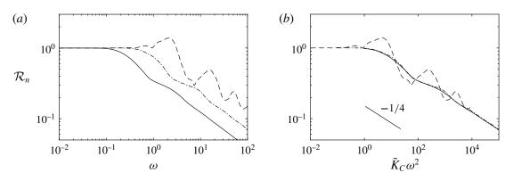
FIGURE 10. Shear reconfiguration number in the convective regime against (a) the frequency ratio  $\omega$ , (b) the rescaled parameter  $K_C \omega^2$ , for  $K_C = 10^0$  (---),  $K_C = 10^1$  (---),  $K_C = 10^2$  (----).
