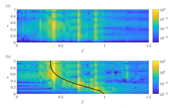
Figure 5.6: Spanwise distribution of power spectral density of (a) the structural motion Y and (b) the wake oscillator q, for  $\Lambda = 10^3$  and v = 49.0. The natural shedding frequency  $f_w^0(s)$  given by the Strouhal law is superimposed in (b) (---).
