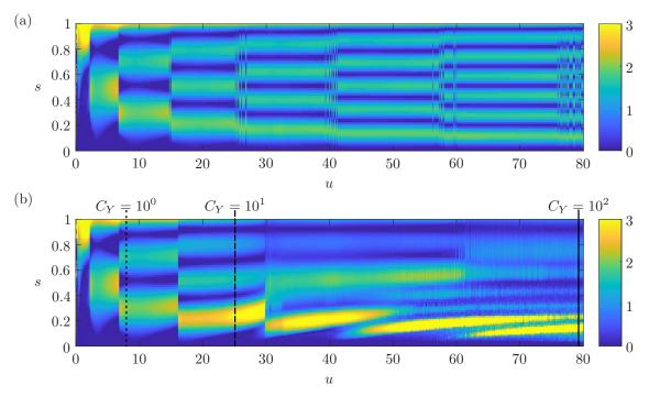
Figure 8: Comparison of the spanwise distributions of energy transfer from the wake to the structure between (a) the straight case and (b) the deflected case  $\Lambda = 10^3$ , for varying reduced velocities u. The colorplots show the mean work of the oscillating lift force  $\langle e \rangle$  normalized by the total energy transfer E. The particular values of the reduced velocity u corresponding to Fig. 2 are indicated as well.
