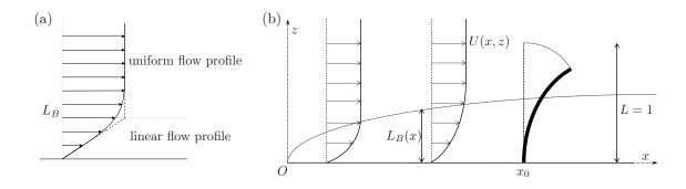
Figure 2.4: Description of the reconfiguration in a Blasius boundary layer. (a) Blasius profile U(x, z) at a fixed x. (b) Beam deforming in a Blasius boundary layer.
