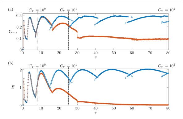
Figure 5.7: Comparison of (a) the RMS amplitude of vibration  $Y_{rms}$  and (b) the total energy transfer E from the wake to the structure, between the straight case (blue  $\circ$ ) and the deflected case  $\Lambda = 10^3$  (orange  $\nabla$ ) for varying reduced velocities v. The particular values of the reduced velocity v corresponding to Fig. 5.2 are indicated as well.
