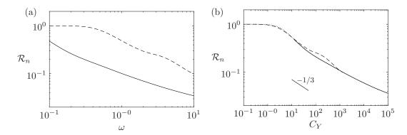
Figure 3.11: Shear reconfiguration number in the large-amplitude regime for  $\lambda = 12.7$ , against (a) the frequency ratio  $\omega$ , (b) the Cauchy number  $C_Y$ , for  $\alpha = 10^0 (--)$ ,  $\alpha = 10^1 (-)$ . Static solution obtained with Eq. (3.21) (····, on (b) only).
