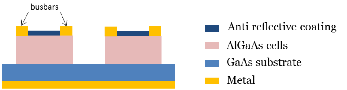
Figure 5.4 - Cross-section schematic of the targeted device after process
