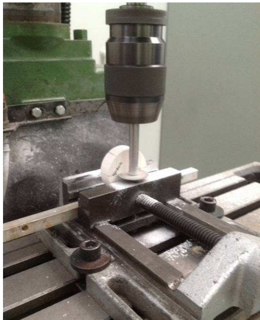
Figure 2. 17 – Notch manufacturing method used in this work – saw of Navier laboratory
