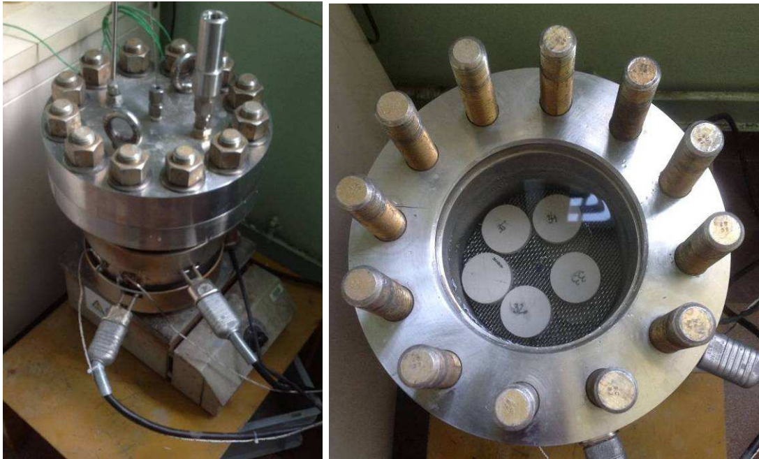
Figure 3. 7- Autoclave IFSTTAR – rock diameter 50 mm
