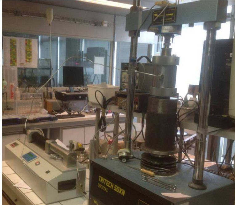
Figure 2. 60 - Cell installed at the press – GDS – dispositive at CERMES
