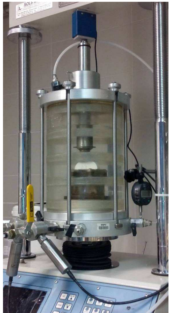
Figure 3. 9- Experimental setup for SCB experiments under confinement in presence of water and CO 2 -saturated water
