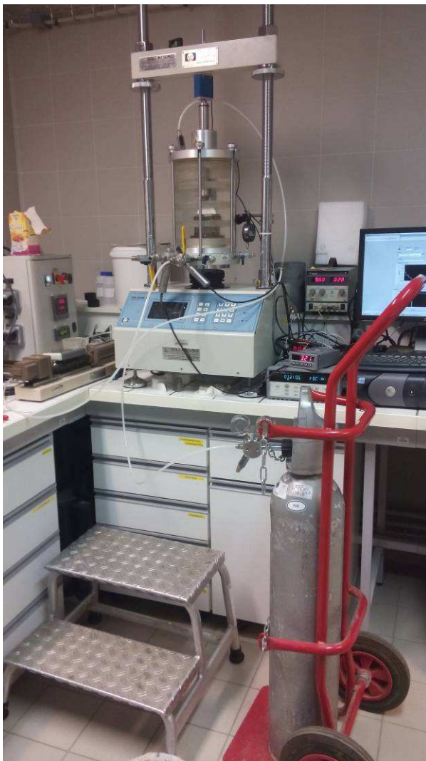
Figure 3. 9- Experimental setup for SCB experiments under confinement in presence of water and CO 2 -saturated water
