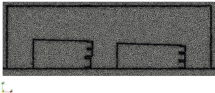
FIGURE 6.37: Cross section along the xz plane with hessian metric
