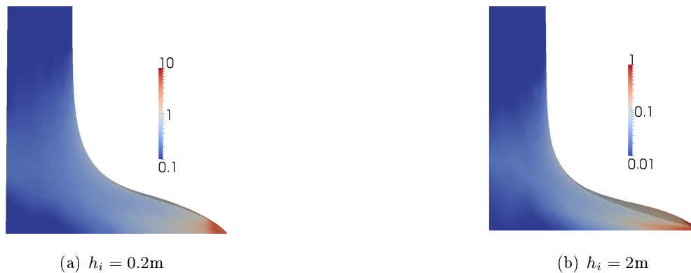
Figure 128: Dense vs. inertial regimes region for time t = \sqrt{h_i/g} , plotted as I/I_0 for granular collapses with a = 10 and different h_i
