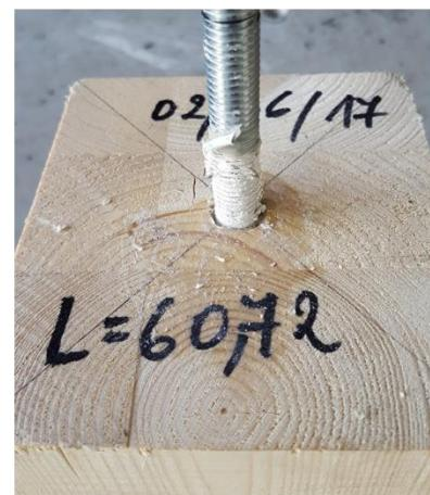
d) Cohesive failure mode at 40°C
