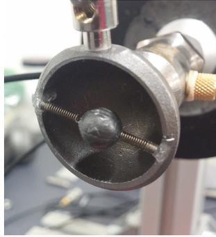
(b) Tested absorber with two springs.
