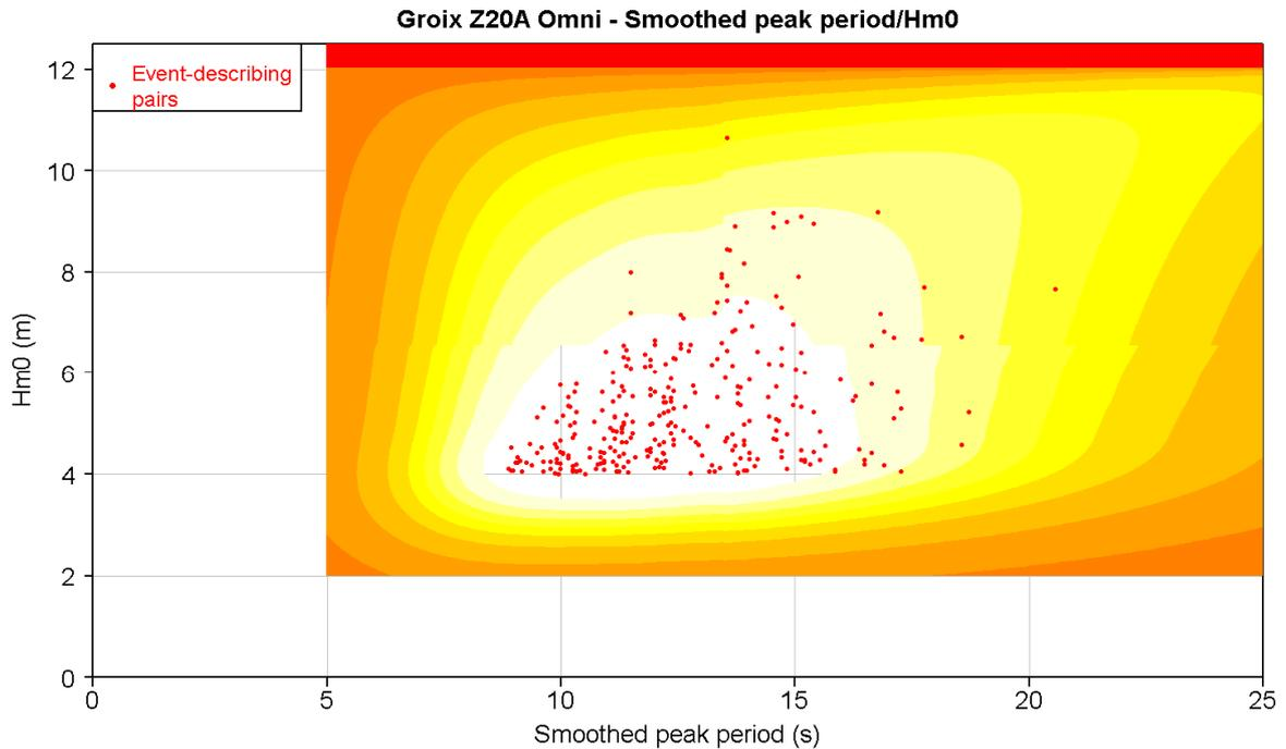
**Figure 42. Joint density  $H_{m0}/T_p$  for event-describing pairs**
