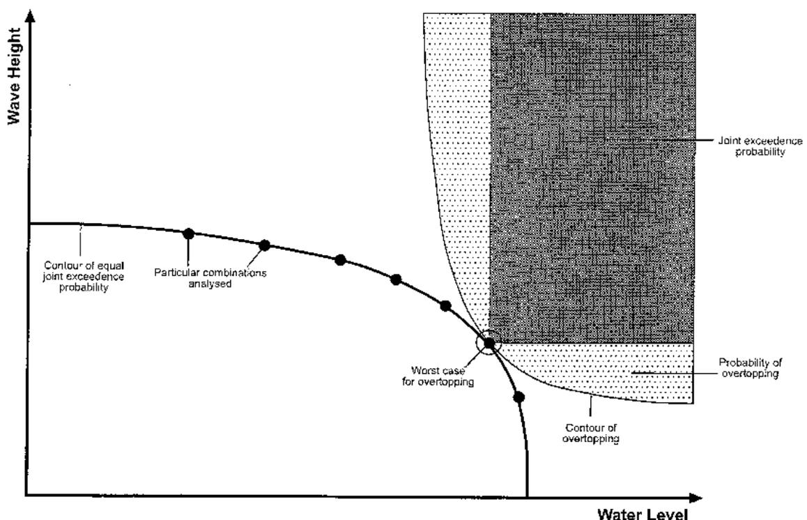
**Figure 38. Joint exceedance probability and structure variable probabilities**
