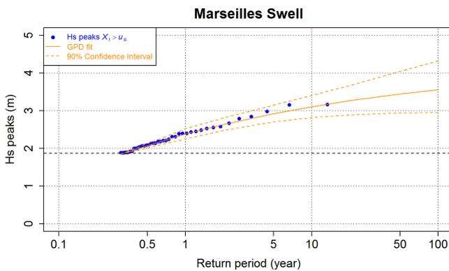
Fig. 4. GPD fit for the swell off Marseille.
