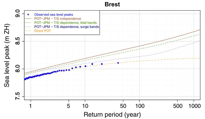
**Fig. 10.** Return levels for sea level events. From the upper to the lower curve: indirect approach without tide–surge interaction, indirect approach with equi-probable tidal bands, indirect approach with equi-probable surge bands, direct approach.
