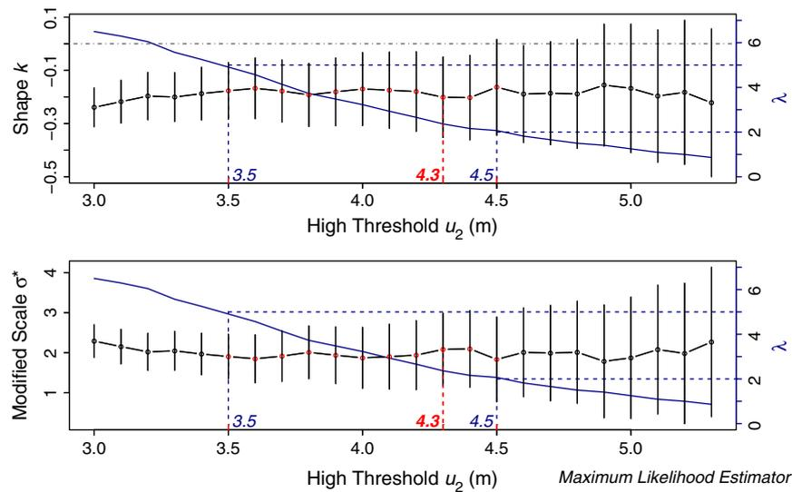
Fig. 3. Gibraltar dataset: stability of shape (above) and modified scale (below) parameters for Generalized Pareto Distribution.
