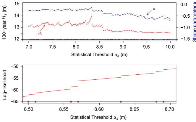
**Fig. 3.** Haltenbanken – change in the ML-estimated GPD shape parameter (top plot, above curve), in  $H_{s100}$  (top plot, below curve) and in the log-likelihood (down plot, zoom) with respect to  $u_s$ . Points represent the data values  $X_{i;N_T}$ .
