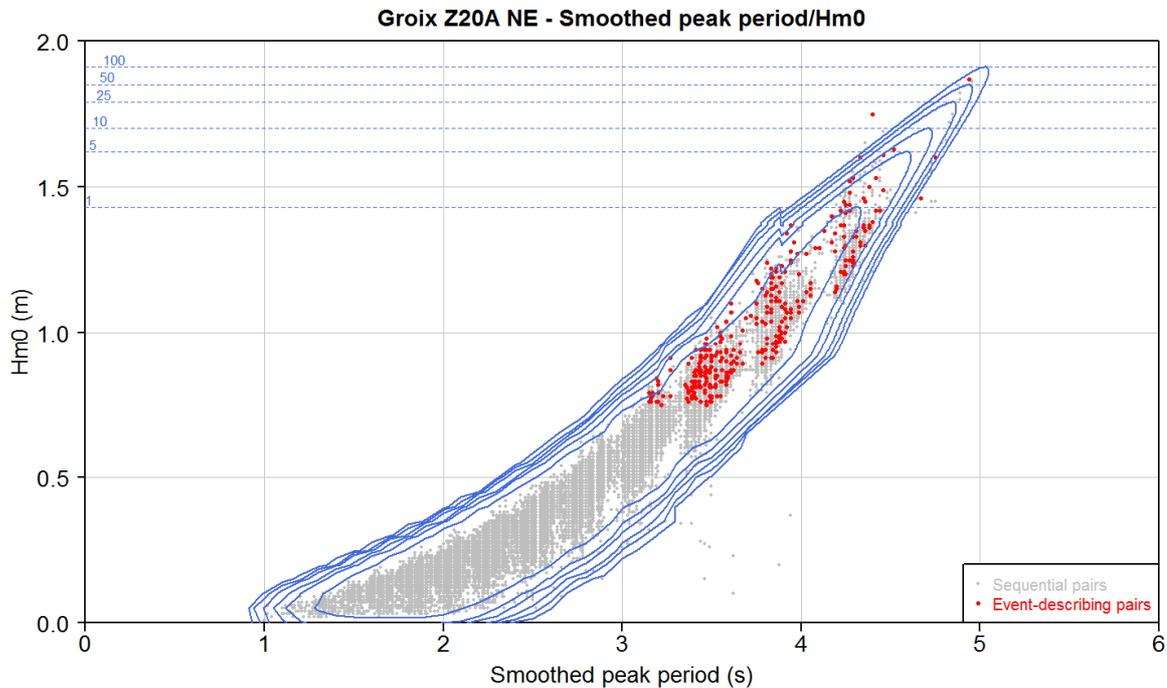
**Figure 46. Contours of sequential  $H_{m0}/T_p$  density associated with extreme  $H_{m0}$  peaks for a homogeneous directional sector**
