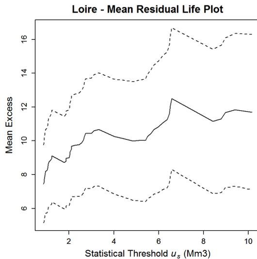
**Fig. 7.** Mean residual life plot for the flood volumes of Loire river sample.
