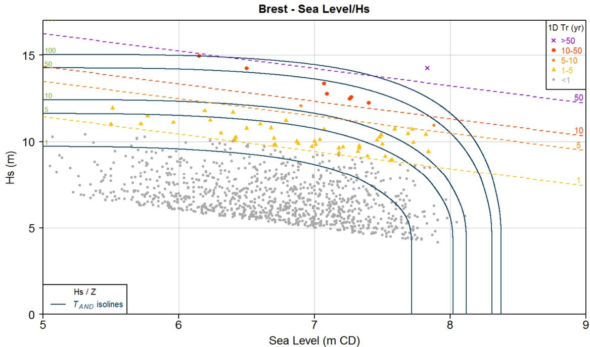
**Figure 39. Contours of joint exceedance probabilities and lines of equal univariate return period of the response function (total water level)**
