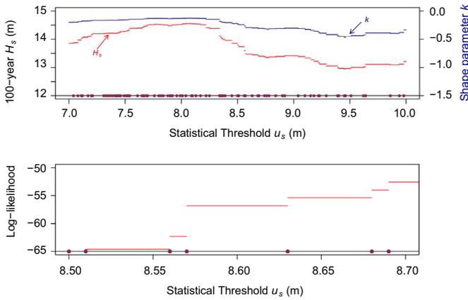
**Fig. 7.** Haltenbanken – change in the L-moments estimated 3-parameter GPD shape parameter and in  $H_{s100}$  (above) and in the log-likelihood (below, zoom) with respect to  $u_s$ . Points represent the data values  $X_{i:N_T}$ .
