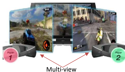
Figure 37 : multi-view screen can give two 3D views because of the High frequency (240Hz) (Sibecas and Eaton, 2012)
