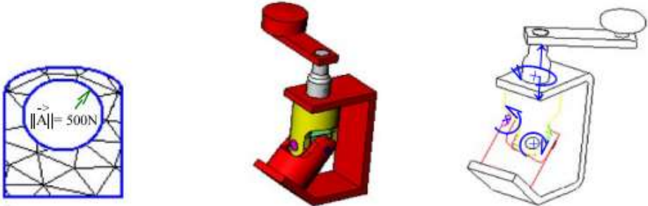
Figure 17 : Master model based approach which contains FEA, CAD and kinetics representations (Bettaieb and Noël, 2008).
