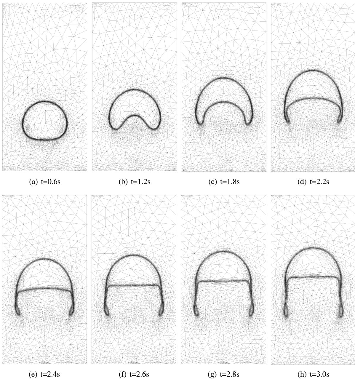
Figure 5.17: 2D rising bubble: Case #2 mesh (10000 elements) at different times.
