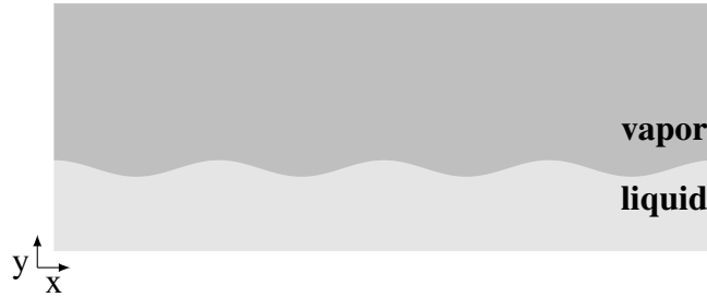
Figure 2.6: Setup for the 2D Rayleigh-Taylor instability. A light fluid lies below a heavy fluid.
