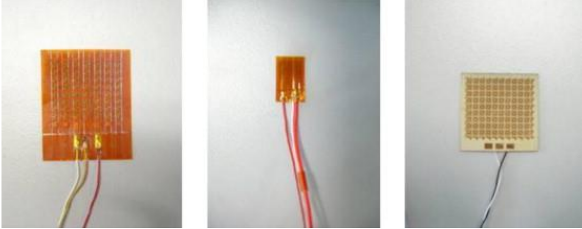
Figure 2.1. Example of heat flux sensors used to measure compressor heat fluxes in the work of Dutra & Deschamps (2013)
