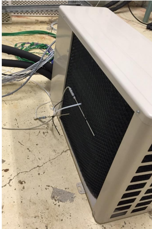
Figure 5.8. Temperature sensor (PT100) used to measure the evaporator inlet air, i.e. T_{ext}
