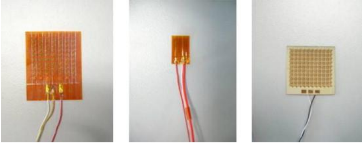
Figure 2.1. Example of heat flux sensors used to measure compressor heat fluxes in the work of Dutra & Deschamps (2013)
