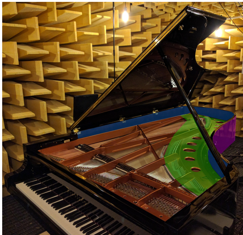
Figure 8.1: A Bösendorfer VC280-9. Highlighted green, blue and purple areas are the surfaces considered in the OTPA for frame, inner rim and outer rim respectively. Note that there are four beams at the frame that terminates at the keyboard end which splits the key range into 5 parts.
