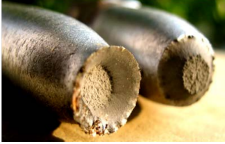
Figure 5.15: Photo produced by [107] showing cup cones fracture in a post mortem ing shear dominating fracture in a post mortem rounded bar.
