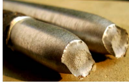
Figure 5.15: Photo produced by [107] showing cup cones fracture in a post mortem ing shear dominating fracture in a post mortem rounded bar.
