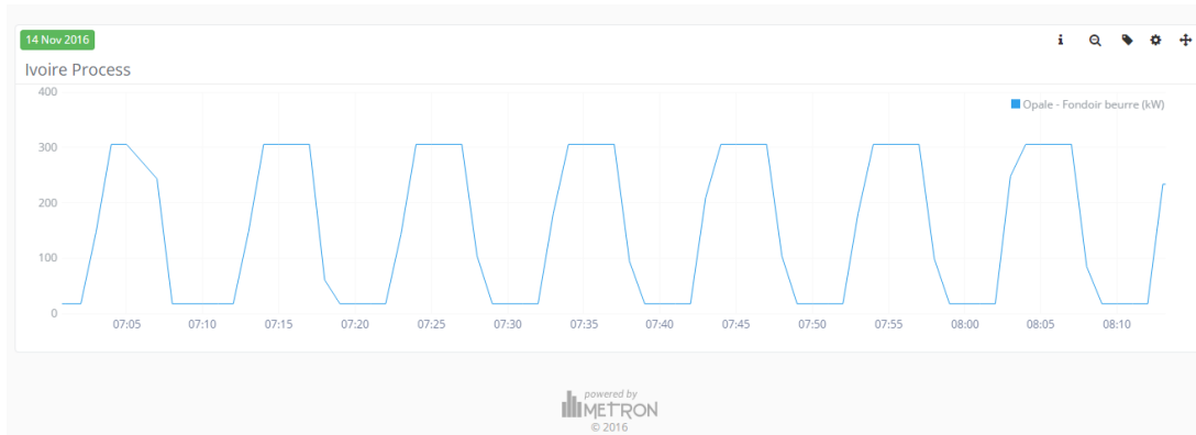
Figure 4.13 – A real power consumption of a typical production process from METRONLab server.
