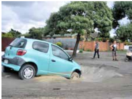
Figure 6.30 – Soil liquefaction caused by the earthquake.
