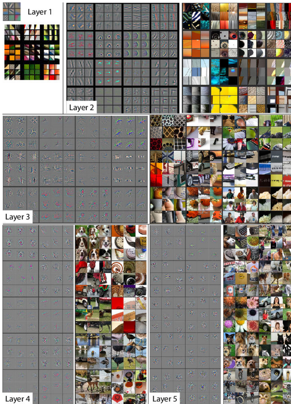
Figure 2.6: Visualization of what activates the most each neuron in a CNN trained for classification on ImageNet 2012 training set, for different layers. Each image on the left contains reconstructed patterns from the validation set of ImageNet 2012 that cause high activations in a given feature map. On the right, the corresponding image patches for each feature map are shown. Figure by Zeiler and Fergus [128].
