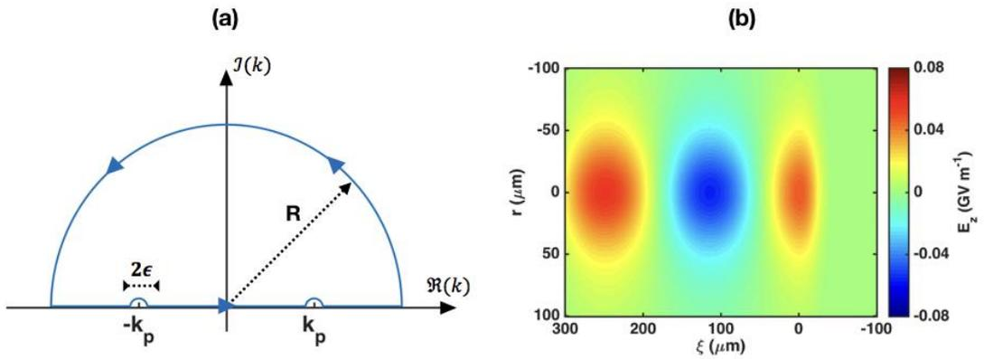
Figure 3.3: (a) Contour  $\gamma$  for the calculation of  $p.v. \int_{-\infty}^{+\infty} \frac{ik k_p^2}{k^2 - k_p^2} e^{ik\xi} dk$ . (b) Longitudinal electric field in the wakefield in the linear regime of a positron driven plasma wakefield. Parameters are  $n_0 = 10^{16} \text{cm}^{-3}$ ,  $N = 10^8$ ,  $\sigma_z = 15 \mu\text{m}$ ,  $\sigma_r = 20 \mu\text{m}$ .
