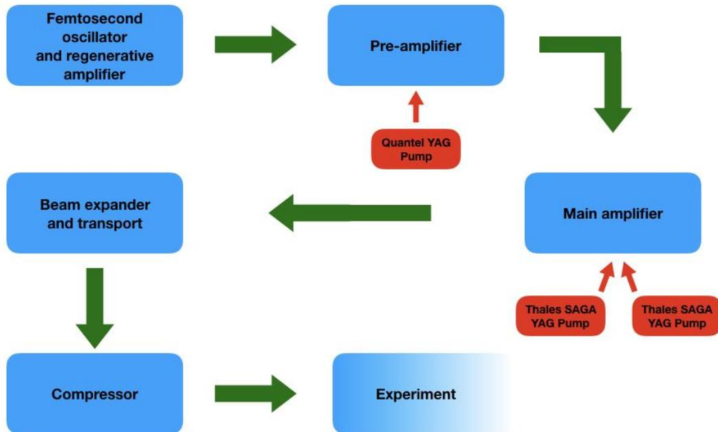
Figure 4.6: Schematic of FACET femtosecond laser systems
