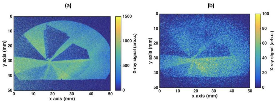
Figure 7.5: (a) X-ray signal on the CCD chip, parameters for this shot were  $P_1 = 17$  bars and  $P_2 = 40$  bars (highest signal in Fig.7.4). (b) X-ray signal on the CCD chip, parameters for this shot were  $P_1 = 17$  bars and  $P_2 = 0$  bars (reference signal in Fig.7.4).
