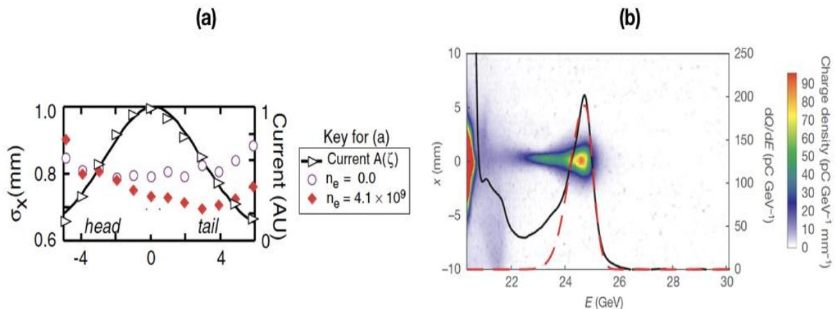
Figure 4.2: (a) Transverse size in  $x$  of the bunch after the plasma. Red squares are with plasma, white circles are without plasma. A strong focusing of the tail occurs. From [Hogan 03]. (b) Accelerated positron bunch in a self-loaded positron PWFA experiment. From [Corde 15].
