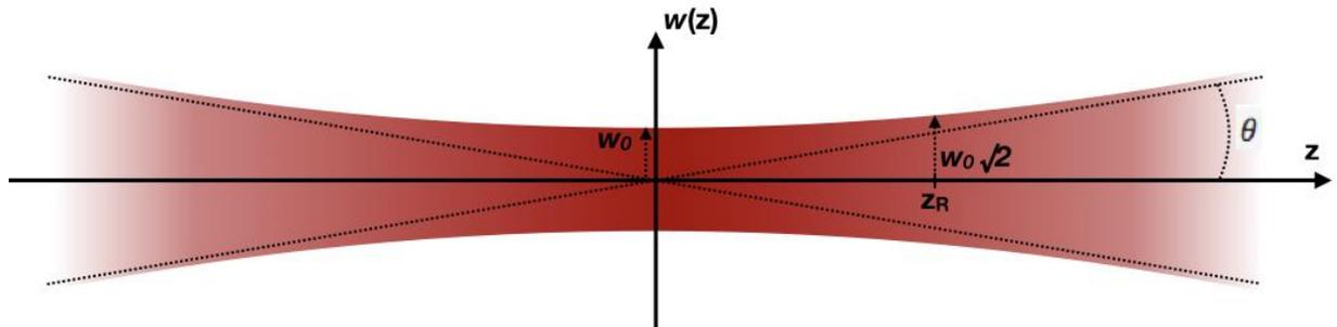
Figure 1.5: A Gaussian beam, near its focus. The plot represents the waist dimension, as a function of the position  $z$ . The meanings of the parameters  $w_0$ ,  $\theta$  and  $z_R$  are also visible.
