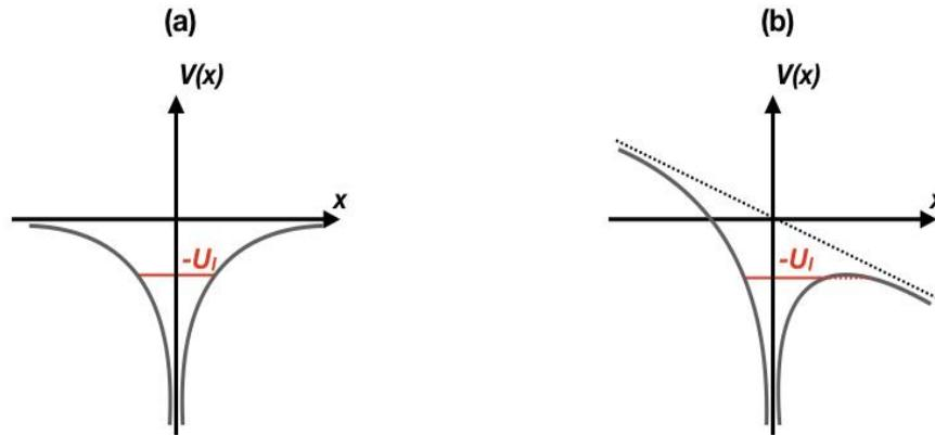
Figure 2.3: Ionization processes (a) Coulomb potential of an atom, the valence electron has an ionization energy  $U_I$ . (b) Tunnel Ionization, when the laser field is strong enough the potential is tilted and makes the tunneling effect (transition through the barrier depicted with a red dashed line) possible. For extremely strong fields, the potential bends enough to permit the suppression of the potential barrier.
