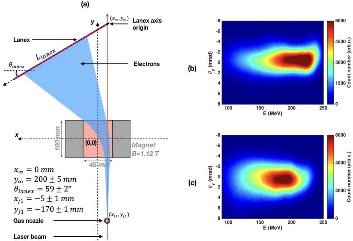
Figure 6.6: (a) Schematic of the spectrometer system. (b), (c) Examples of electron bunch spectra measured by the spectrometer. The images were processed: the energy axis is established thanks to a code which calculates the trajectories of the electrons in the field of the magnetic dipole.
