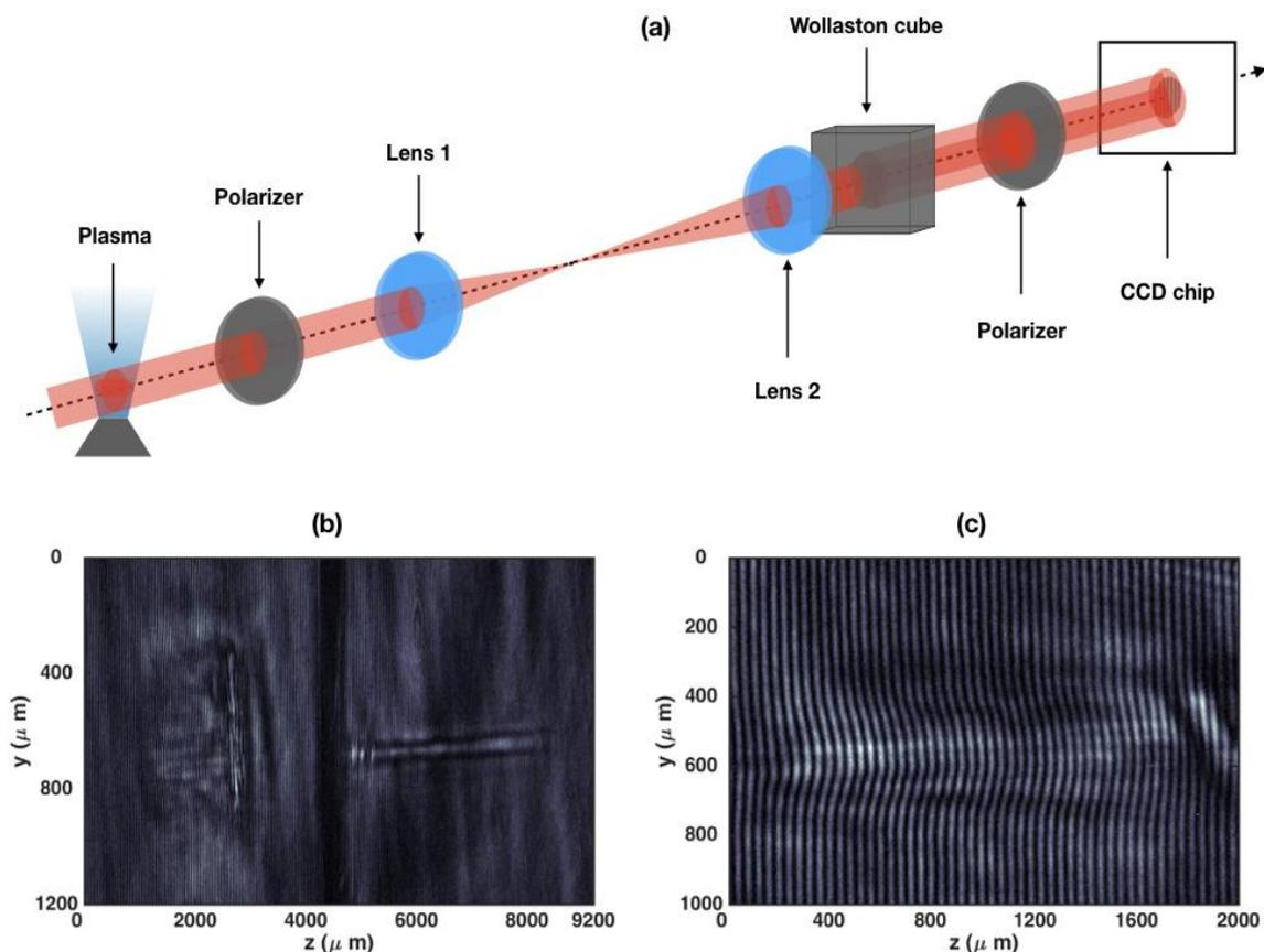
Figure 6.7: (a) Schematic of the side-view diagnostic. (b) Example of an image recorded on the camera. On the left, a plasma wakefield is created in the first jet (nozzles are not visible). The wheel intercepts the laser beam (center), and the electron beam ionizes a thin column of gas in the second jet (on the right). (c) Perturbations of fringe spacing in both jets allows to retrieve the plasma density.
