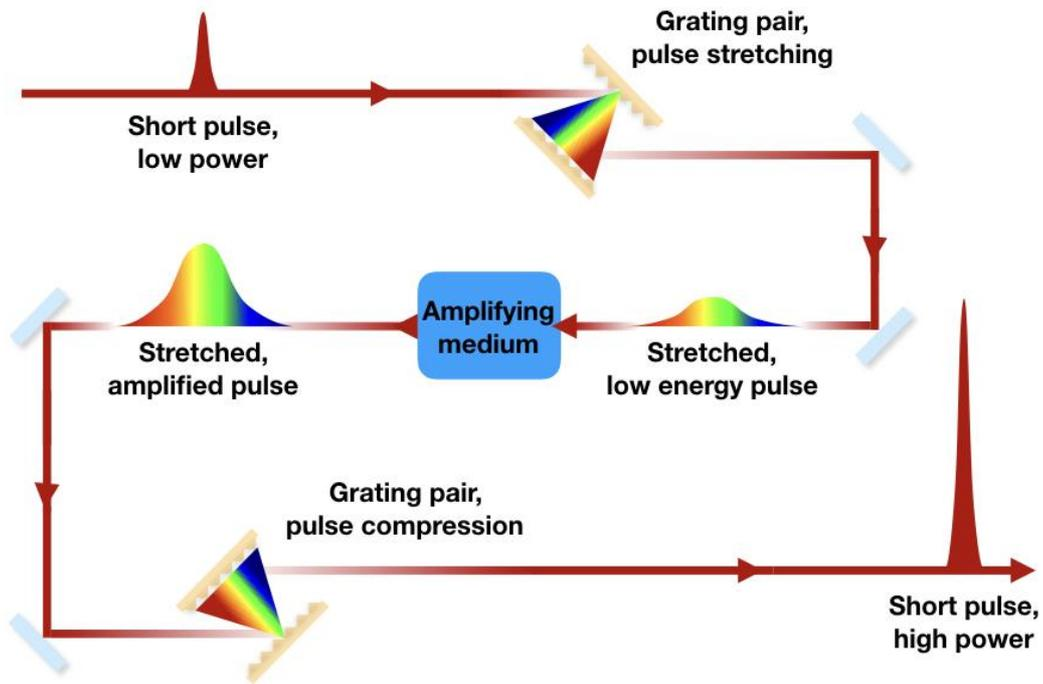
Figure 1.6: Schematic of the chirped pulse amplification technique.
