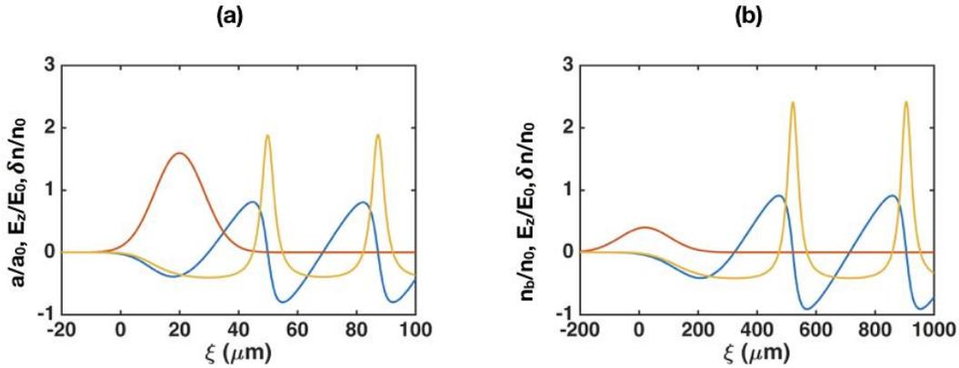
Figure 3.5: (a) Laser driven nonlinear plasma density wave. (red) Laser field ( $a/a_0$ ), (blue) longitudinal electric field on axis ( $E_z/E_0$ ), (yellow) plasma electron density  $n_p/n_0$  ( $a_0 = 2$ ). (b) Electron beam driven nonlinear density wave. (red) Beam Current  $n_b/n_0$  (blue)  $E_z/E_0$  field on axis, (yellow) plasma electron density  $n_p/n_0$ . ( $n_0 = 10^{16} \text{cm}^{-3}$ ).
