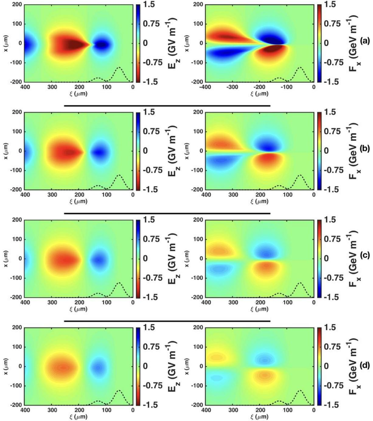
Figure 5.13:  $E_z$  field map (left) and transverse force  $F_x$  (right) after 72.5 cm of propagation in the plasma, for the case without spoiling (a), with 100  $\mu\text{m}$  of Titanium (b), with 179  $\mu\text{m}$  of Titanium (c), with 257  $\mu\text{m}$  of Titanium (d).
