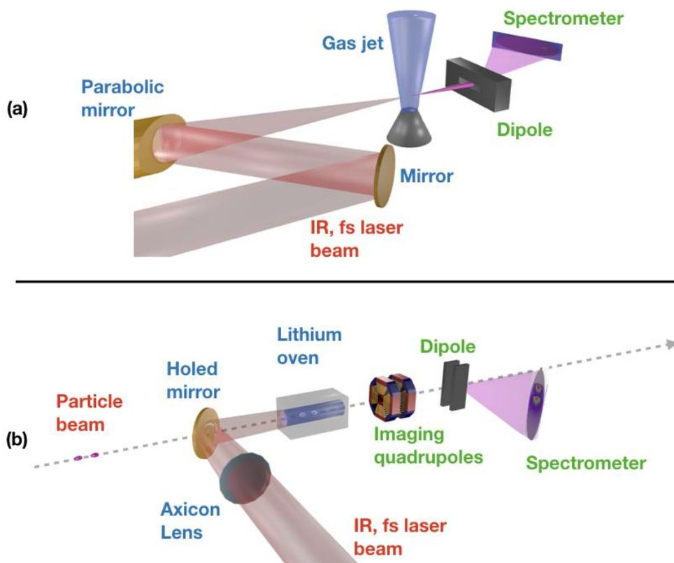
Figure 0.2: (a) A typical laser wakefield experiment, a parabolic mirror focuses a laser beam into a gas jet. The emerging electron beam is characterized by a spectrometer. (b) A plasma wakefield experiment, in which two particle bunches are sent into a laser pre-ionized plasma. A spectrometer displays the energy of the particle bunch emerging from the plasma. This experiment can be carried out with electron or positron bunches.
