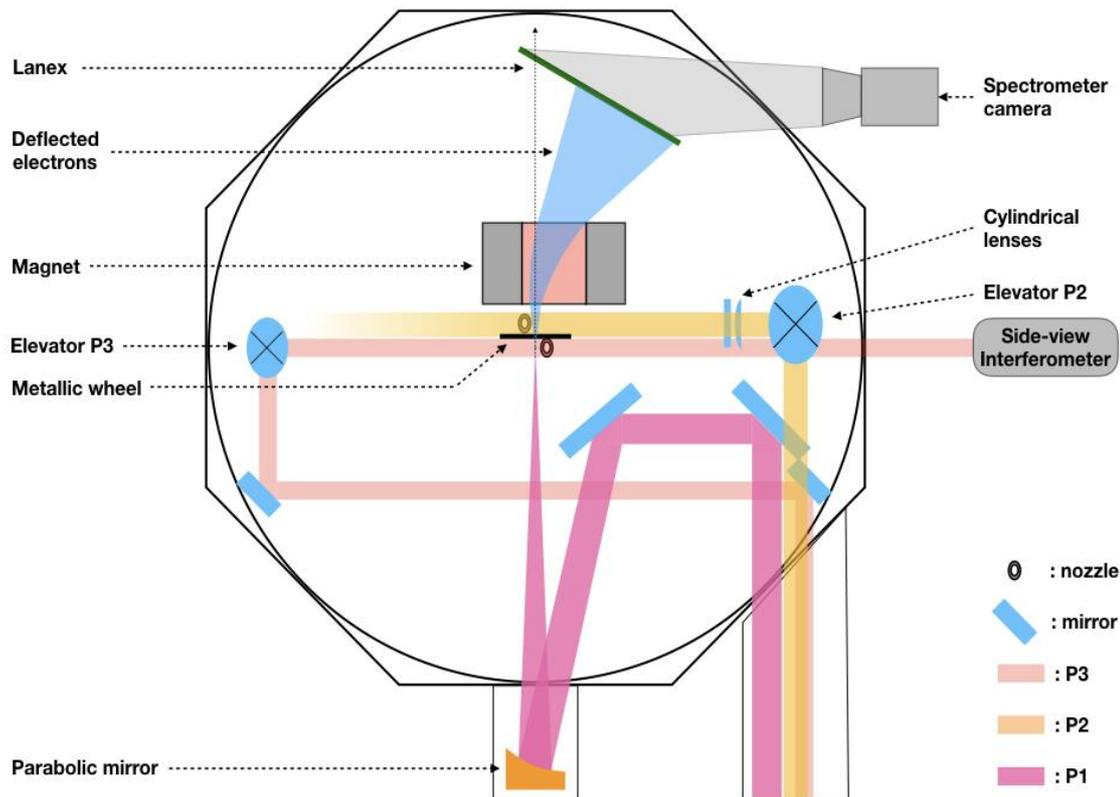
Figure 6.5: Schematic of the hybrid LWFA/PWFA experiment.
