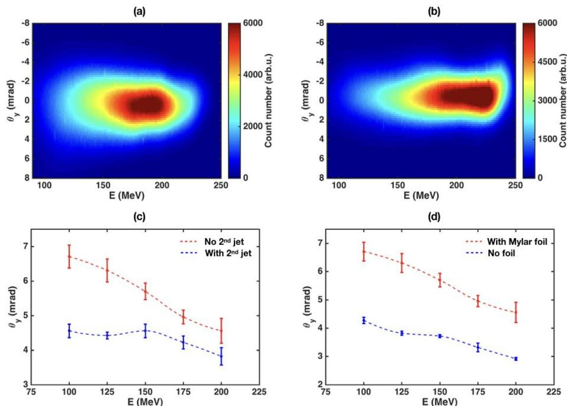
Figure 6.9: (a) Example of an electron bunch spectra, for a shot with a Mylar window to block the laser, but no gas in the second jet. (b) Same, but with gas in the second jet. (c) Divergence of the beam on the spectrometer as a function of the particles energy. The focusing effect of the second gas jet is visible. (d) Divergence of the beam on the spectrometer as a function of the particles energy. This is an evidence of the defocusing effect of the Mylar foil.
