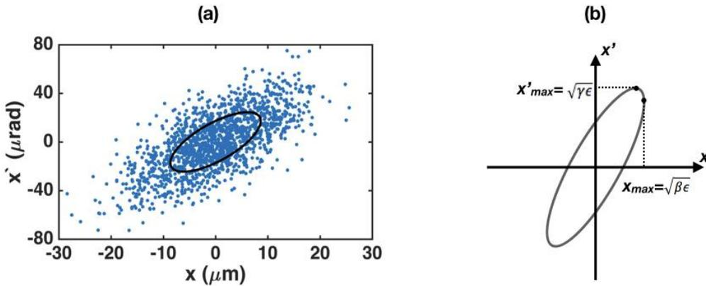
Figure 1.7: (a) Particle distribution in trace-space. The black line is the ellipse whose equation is given above. Its area is  $\pi\epsilon$ . (b) Dimensions of the ellipse expressed with the Twiss parameters.
