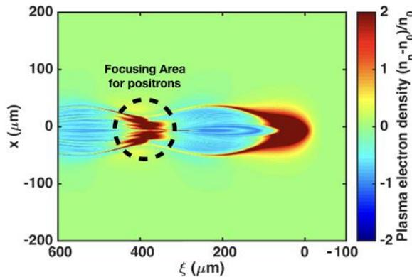
Figure 4.1: Plasma electron density in a positron wakefield from a PIC simulation. The code QuickPIC was used, with  $n_0 = 10^{16} \text{ cm}^{-3}$ , and a drive bunch of charge  $Q_{drive} = 480 \text{ pC}$  and dimensions  $(\sigma_x, \sigma_y, \sigma_z) = (35 \text{ } \mu\text{m}, 25 \text{ } \mu\text{m}, 30 \text{ } \mu\text{m})$ . The focusing and accelerating area is very limited, by contrast, the large blue area is very defocusing for positrons.
