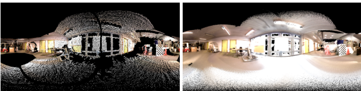
Figure 7.7 – Virtual keyframe fusion example. The left image depicts the initial keyframe. The resulting keyframe after fusion of the nearby frames is shown in the right. Observe that the occlusions are handled using this representation and the final model is a more complete keyframe with a bigger region of interest.
