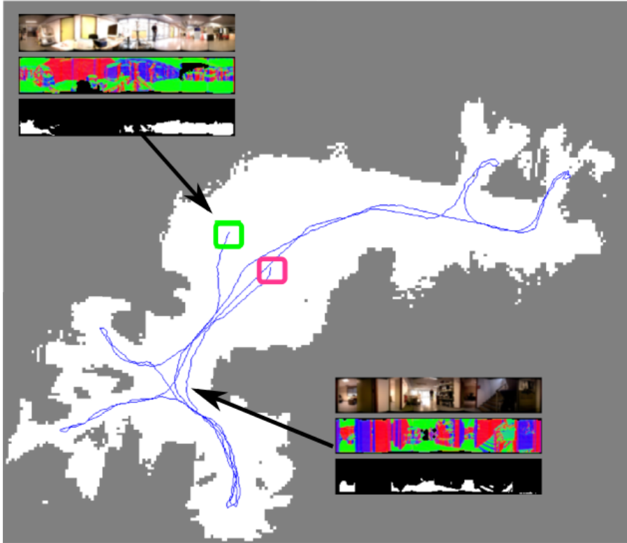
Figure 7.4 – Free space extraction in the real indoor sequence. The camera trajectory starts in the green box and the endpoint is indicated by the red box. The points belonging to the floor in each frame are used to extract the free space. Two examples of the regions of the free space are shown with the RGB and normal images. The accumulated free space grid using the computed trajectory are the regions in white, while the occupied or not explored regions are shown in gray.
