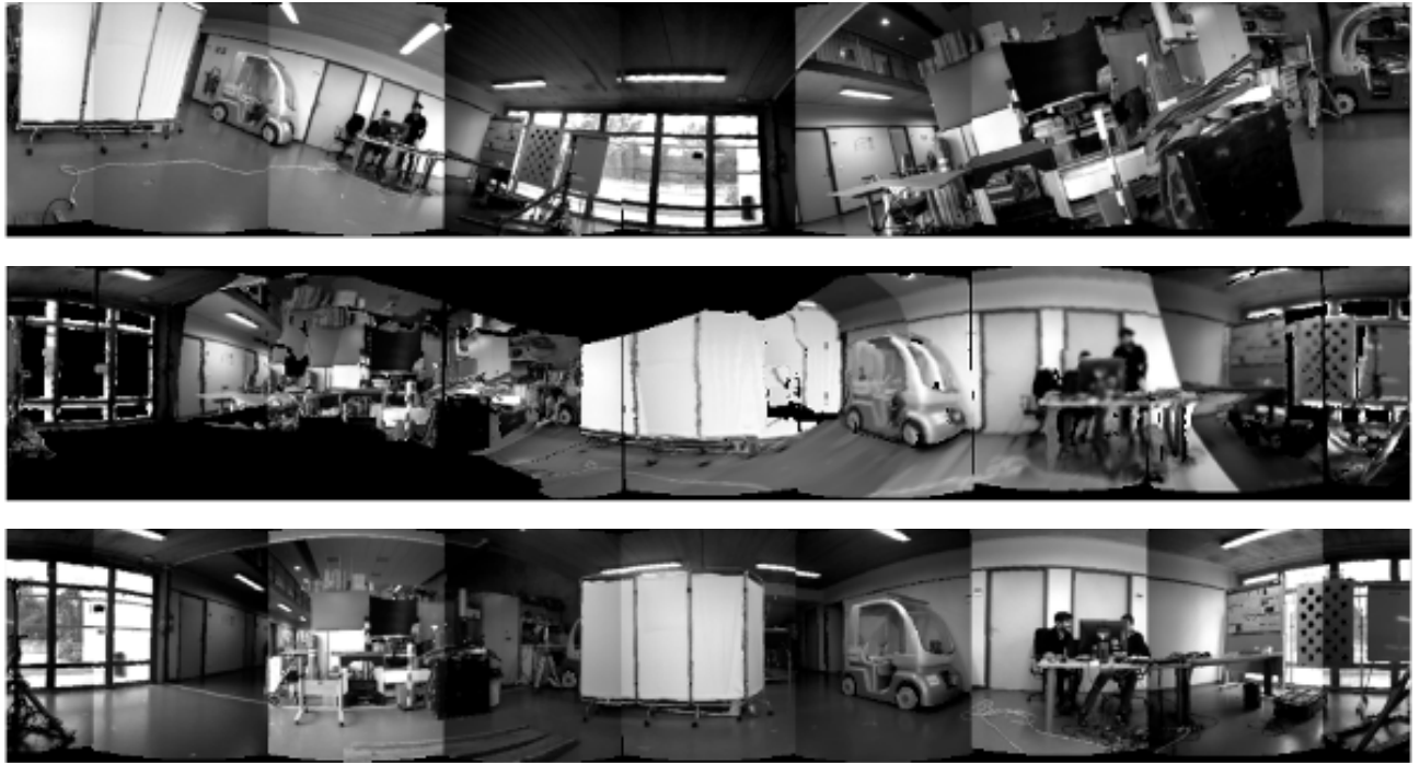
Figure 3.5 – Virtual image rendering example using the spherical warping at a different view-point. The virtual view, shown in the second row, is rendered using the current frame (first image) at the the position of the reference frame (third row).
