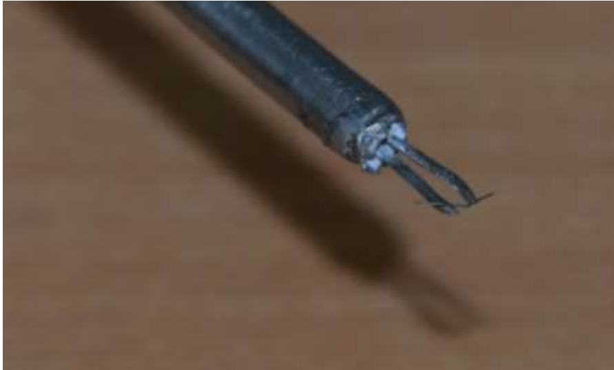
Figure 170 : Micro-thermocouple de 25 \mu m assemblé
