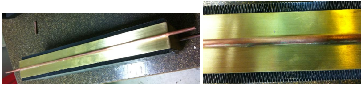
Figure IV-25 – Collage des ailettes externes
