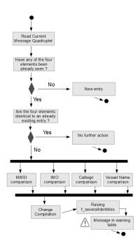
Figure 5.15: Processing of the compliance with the fleet register database
