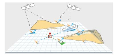
Figure 3.1: Transmissions between AIS stations
