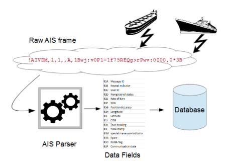
Figure 5.1: Process of AIS message parsing
